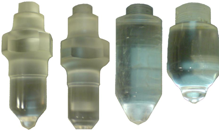
**Figure 3-27: photographs of selected enlarged transparent needle parts used with multi-hole nozzles.**
