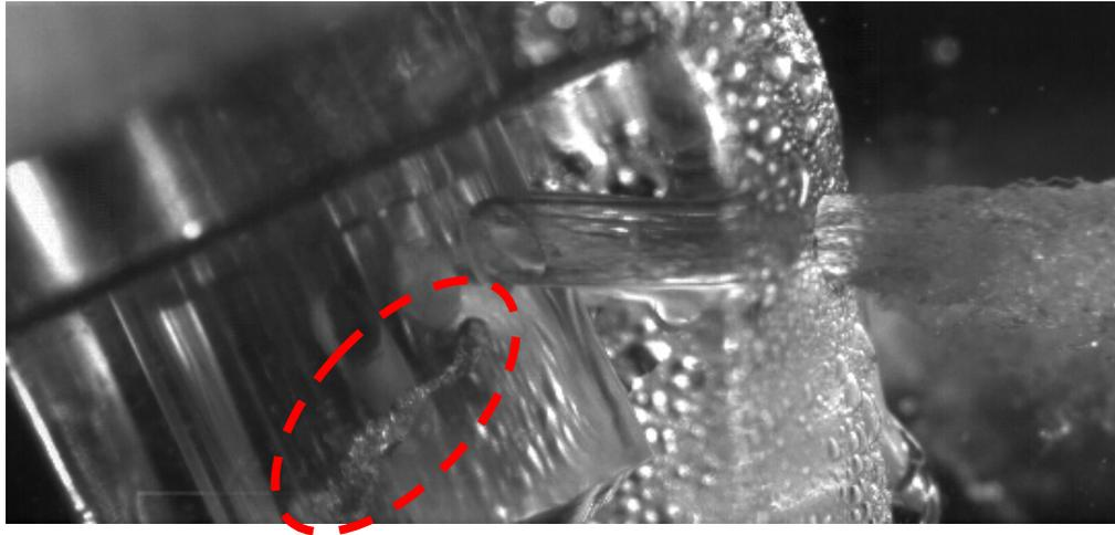
**Figure 6-5:** Image showing string location inside the no-groove five-hole nozzle.
