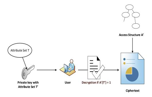
Figure 4.6Ciphertext-Policy Attribute-Based Encryption Scheme
