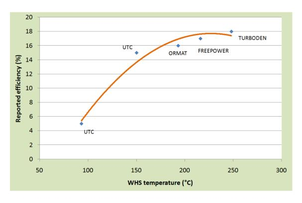
Figure 22 Reported efficiency vs. waste heat source temperature curve for commercial systems
