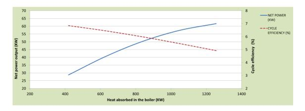
Figure 56 Variation and trade off between power output and cycle efficiency
