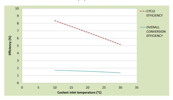
Figure 53 Effect of coolant temperature on cycle and overall conversion efficiency for fixed waste heat
