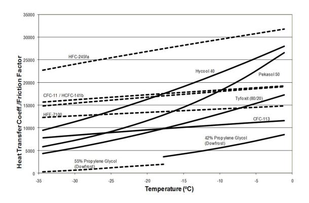
Figure 27 Performance of heat transfer fluids (source: Honeywell)
