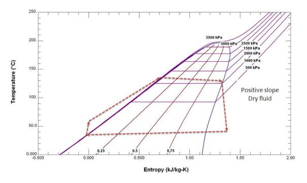
Figure 13 T-S diagram for dry fluids (Pentane)
