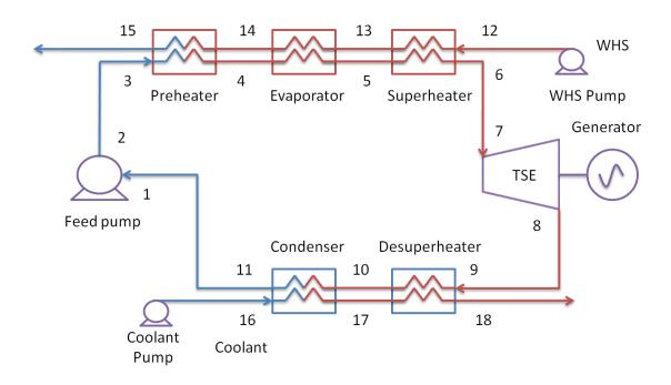
Figure 4 Schematic superheated ORC system layout
