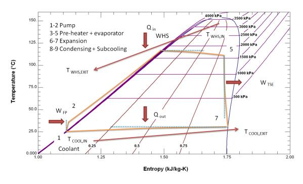
Figure 3 T-S diagram for ORC using R245fa with wet vapour expansion
