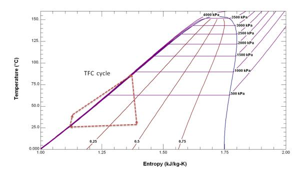
Figure 16 T-S diagram for TFC using R254fa
