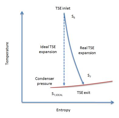
Figure 30 T-S diagram for expander representing losses
