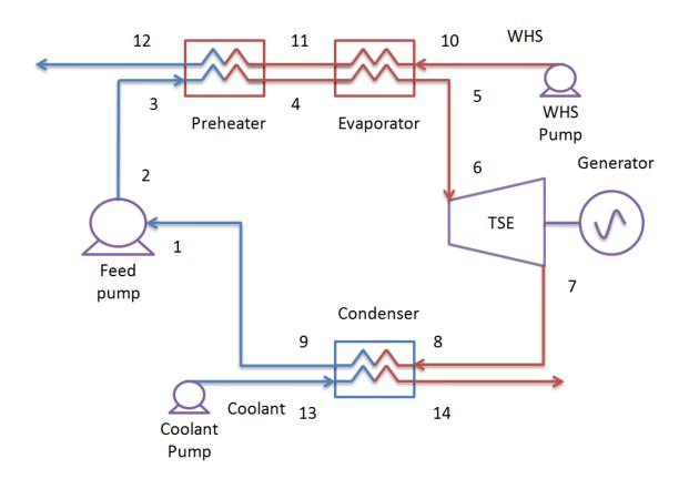
Figure 2 Schematic ORC system layout for wet vapour expansion
