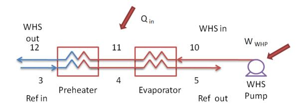
Figure 37 Preheater evaporator layout for simulation analysis
