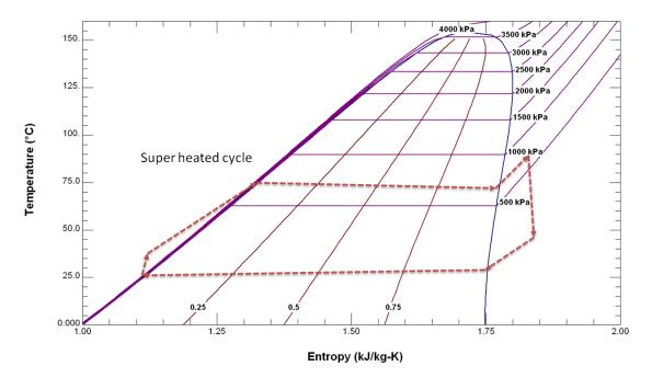
Figure 18 T-S diagram for superheated cycle using R254fa
