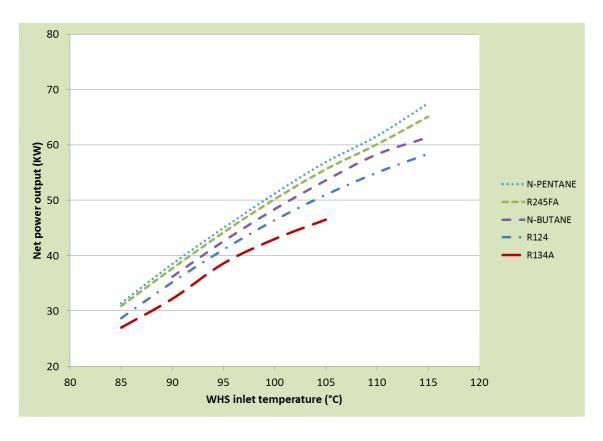
Figure 26 Net power output vs. waste heat source inlet temperature comparison for few working fluids
