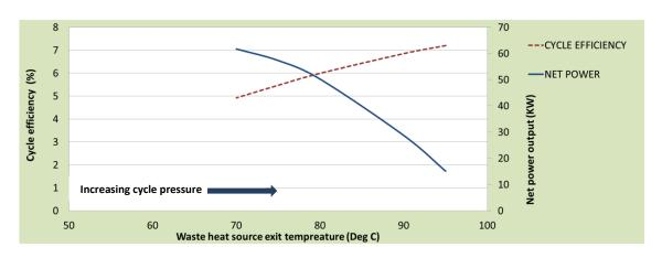
Figure 49 Effect of heat source exit temperature on cycle efficiency and net power out with fixed waste heat inlet condition
