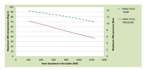
Figure 48 Relationship between maximum working fluid temperature and the amount heat absorbed for fixed waste heat inlet condition
