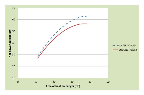
Figure 41 Net power output vs. Heat exchanger area trend for cooling tower and water cooled condensers
