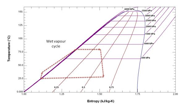
Figure 17 T-S diagram for wet vapour cycle using R254fa
