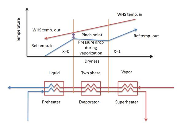
Figure 35 Temperature vs. Dryness change in boiler showing pressure drop
