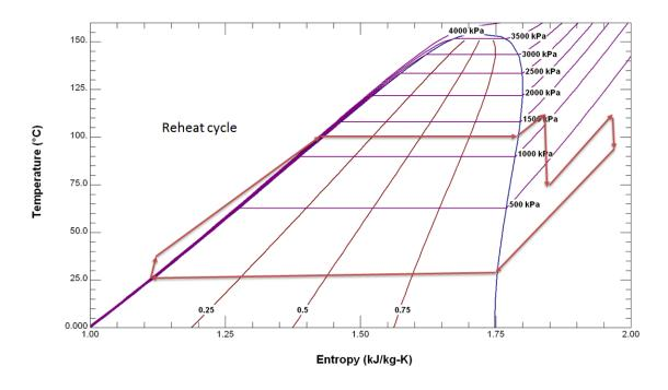
Figure 8 T-S diagram for reheat ORC using R245fa
