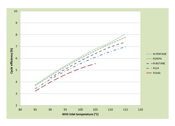
Figure 25 Cycle efficiency vs. waste heat source inlet temperature comparison for few working fluids
