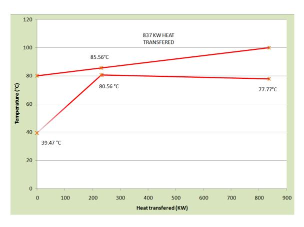
Figure 38 Temperature profile vs. Heat transferred in the preheater and evaporator for the simulated ORC case
