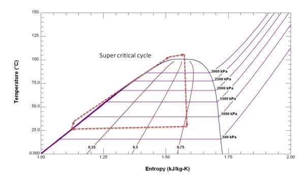
Figure 19 T-S diagram for supercritical cycle using R134a
