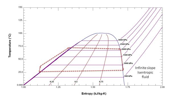
Figure 15 T-S diagram for isentropic fluids (R134a)
