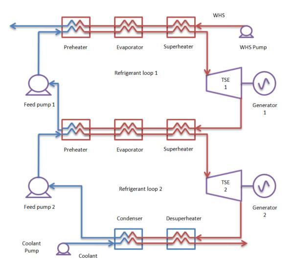
Figure 9 Schematic layout for dual ORC systems
