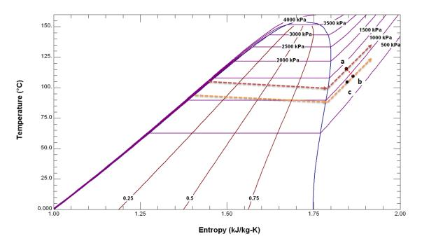
Figure 31 Losses during transporting fluid in the ORC
