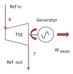
Figure 39 Expander generator layout for simulation analysis
