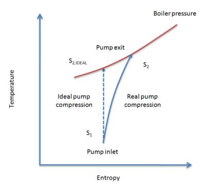
Figure 29 T-S diagram for feed pump representing losses
