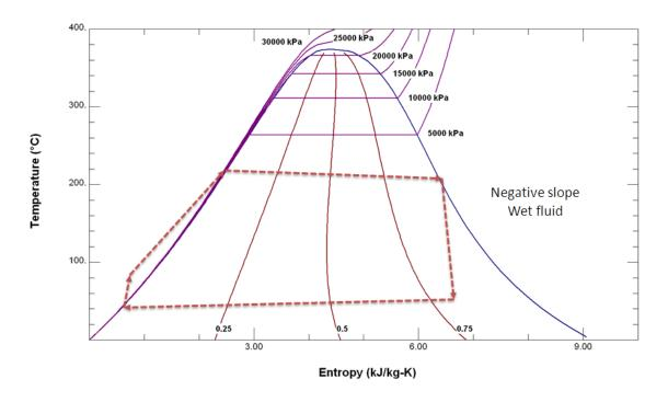
Figure 14 T-S diagram for wet fluids (Water)
