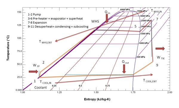
Figure 5 T-S diagram for superheated ORC using R245fa
