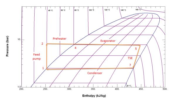
Figure 45 P-h diagram for the simulated cycle
