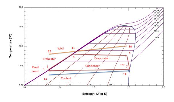
Figure 44 T-S diagram for the simulated cycle
