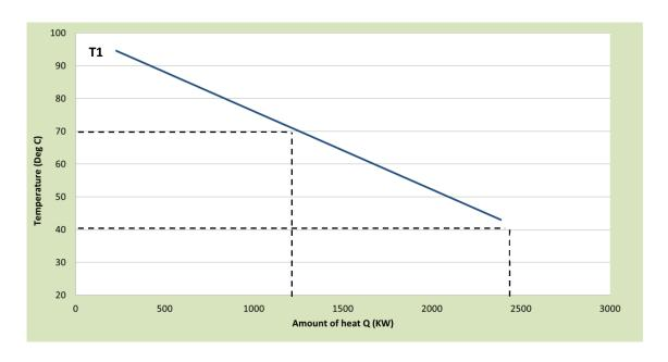
Figure 47 Heat transfer as a function of temperature for single phase heating medium
