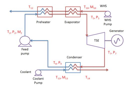
Figure 57 Minimum instrumentation diagram to validate simulation results
