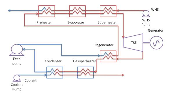
Figure 6 Schematic ORC with a regenerator
