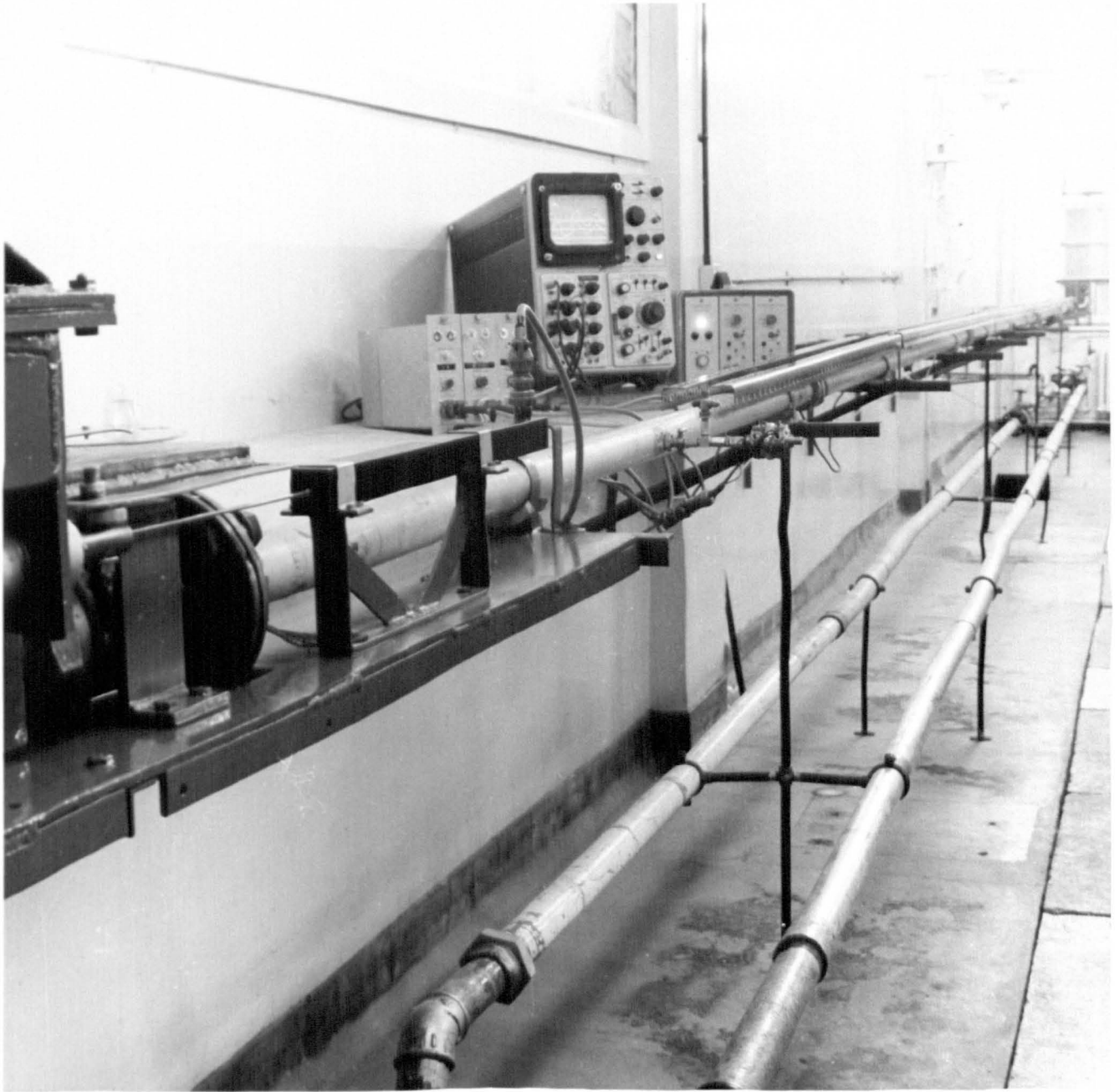
Fig. 22 View upstream from the valve in pipeline configuration 1, illustrating the pipe support brackets.
