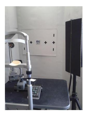
Figure 46. Experimental setup showing the display area, chin rest, and one of two illumination systems
