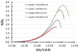
Figure 18. Non-dimensional spread factor from WFM simulation plotted against non-dimensional time for hydrophilic surfaces.  $\theta_{adv}$ = 10°-70°. We=0.2-117, x-axis, logarithmic scale.
