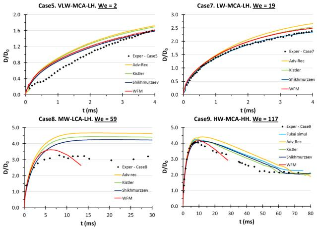
Figure 14. Comparison of WFM results against experiments and respective simulations for the hydrophilic surfaces of Cases5,7-9 listed in Table 2 (where references can be found); corresponding predictions from other dynamic contact angle models found in literature are also indicated.
