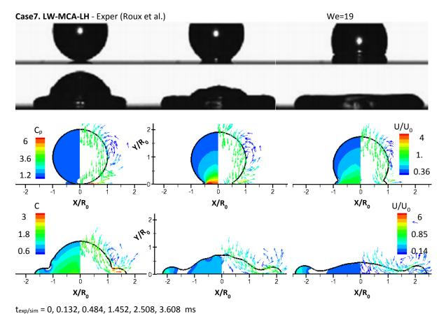
Figure 17. Comparison with experiment for Case7 LW-MCA-LH. C<sub>p</sub> contour and velocity vectors colored by velocity magnitude are plotted. C<sub>p</sub> values below 0.01 are cutoff. The first contour legends apply to the first 3 pictures, while the second one applies to all the other.
