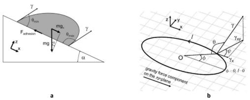
Figure 1. Adhesion force. a) Droplet sliding down an incline. At the moment it starts moving,  $F_{adhesion} = mg \sin a$ . b) Projection of the contact area of the droplet on the incline. Both Images taken from Antonini et al. [75]
