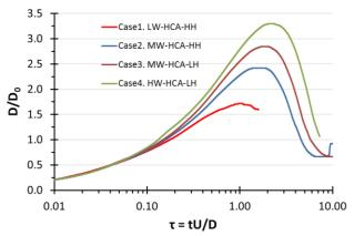
Figure 13. Non-dimensional spread factor from WFM simulation plotted against non-dimensional time for hydrophobic surfaces.  $\theta_{adv}$ = 105°-120°. We=8-91, x-axis, logarithmic scale.
