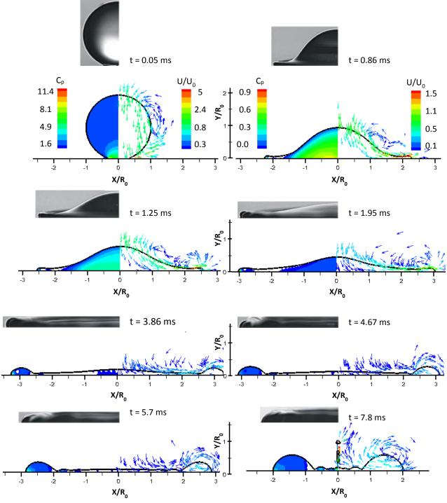
Figure 12. Comparison with experiment for Case4. HW-HCA-LH (Sikalo et al. [50]). Pictures taken from reference. Cp contour and velocity vectors colored by velocity magnitude are plotted. Cp values below 0.01 are cutoff. The first contour legends apply to the first picture, while the second one applies to all the other.
