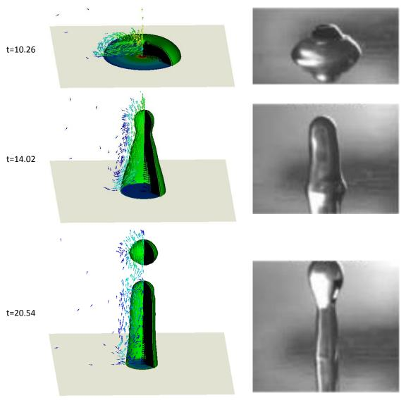
Figure 11. Comparison with experiment for Case 3. MW-HCA-LH (Rioboo et al. [30]). Pictures taken from reference. Results are represented in 3 dimensions, after the revolving of symmetry axis.  $C_p$  contour and velocity vectors colored by velocity magnitude are plotted.  $C_p$  values below 0.01 are cutoff. The first  $C_p$  contour legend applies to the first two pictures, while the second one applies to all the following. Velocity contour is the same for all pictures.
