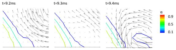
Figure 4. Unphysical diffusion of volume fraction field, followed by the breakup of small secondary droplet observed when the Wetting Force is applied in a wide region around the contact line. Velocity vectors are plotted in the same manner for all pictures. The numerical tests have been performed for the conditions of Case 9.
