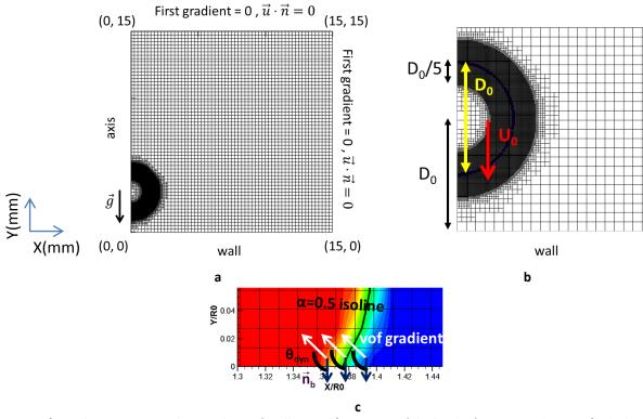
Figure 5. a) Initial Domain + Boundary conditions for all cases, b) Depiction of the local refinement technique, c) calculation of  $\theta_{dyn}$  for the WFM.
