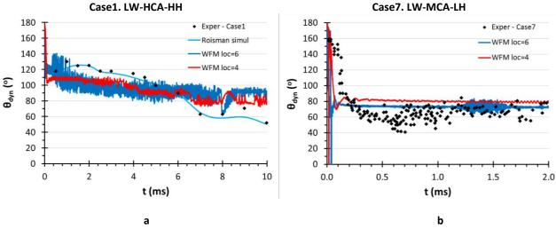
Figure 6. Effect of grid size for Cases 1. LW-HCA-HH and 7. LW-MCA-LH of Table 2 a)  $\theta_{dyn}$  as a result of the WFM simulation using 4 and 6 levels of local refinement in comparison with the experimental values and simulation results of Roisman et al. [41]. b)  $\theta_{dyn}$  as a result of the WFM simulation using 4 and 6 levels of local refinement in comparison with the experimental values of Roux et al. [40]. The symbol "rm" in the graphs stands for remeshing.
