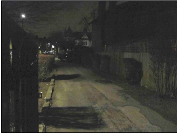
Figure 3.7. An observers' view of the night-time residential scene used in the measurement of discomfort glare thresholds. The glare source was presented through an aperture in the centre of the image. Small red fixation spots were positioned at -0^\circ , -3^\circ , -6^\circ and -12^\circ to aid peripheral fixation.
