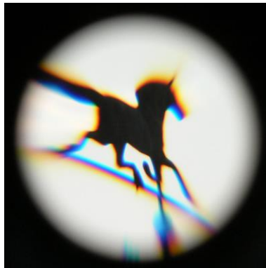
Figure 1.11. Example of a chromatically aberrated image.
