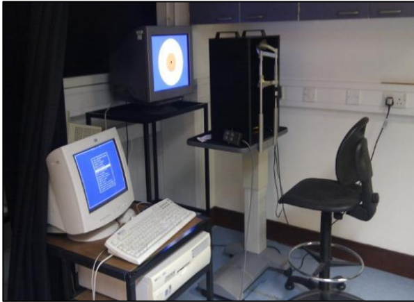
Figure 3.3. The experimental setup for the flicker cancellation technique. The display in the foreground of the photo is used to set up and control the experiment, while the participant is seated on the right and views the far display through the hood.
