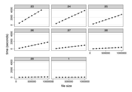
**Figure 4**: Query time in seconds for finding each nearest neighbor by a Multibit Tree (C++ version) in a file with 1 million records for varying file sizes (200.000 - 1.000.000) depending on the similarity threshold (.93 - 1).
