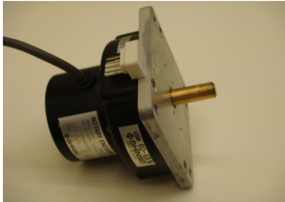
Figure 8.5 A Photo of Piezoelectric Ultrasonic Motor by Shinsei USR60E3N.
