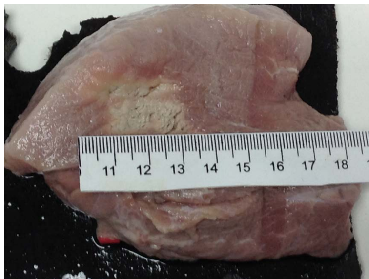
Figure 10.18 Photograph of the overlapping thermal lesions created in pork tissue in vitro using both linear and angular stages of the positioning device. The ablation grid was 5x5 with spacing between lesions of 2 mm for the linear stage and 3° for the angular stage.
