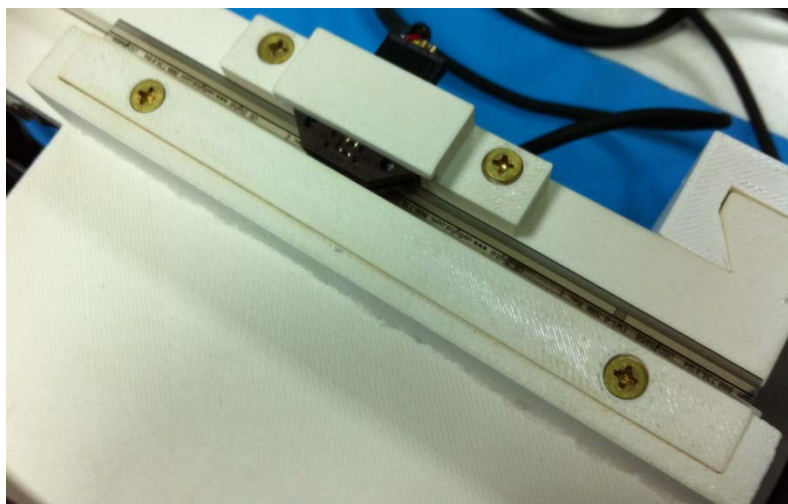
Figure 7.10 A photograph of the installation of the linear encoder module on a strip
