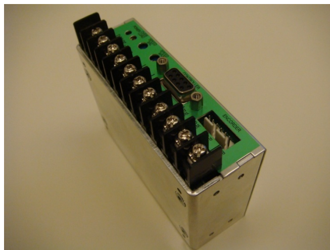
Figure 8.6 A Photo of Dedicated Driver for Shinsei USR60 Series, Shinsei D6060E.
