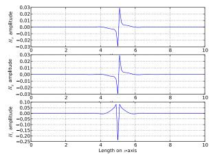
(c) Propagation of **H** field components along *z*-axis
