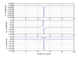
(b) Propagation of **H** field components along *y*-axis
