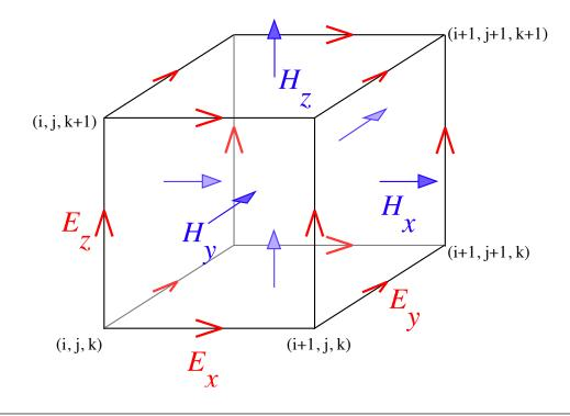
Fig. 1.1 Field component distribution in Yee's lattice in 3D (image taken from Wikipedia)
