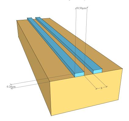
Fig. 10.6 Schematic diagram of the nano directional coupler
