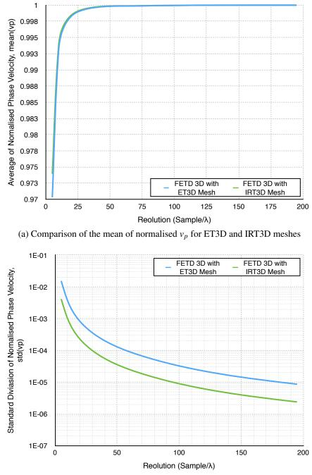
(b) Comparison of the standard deviation of normalised  $v_p$  for ET3D and IRT3D meshes
