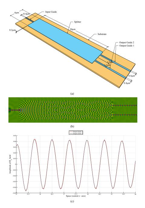
Fig. 10.4 (a) Schematic 3D diagram of the nano power splitter (sky blue part is the *Si* core and orange coloured part is  $SiO_2$  substrate), (b)  $H_y$  field profile at the central *zx*-plane of the power splitter after 9000 time-steps, (c) Comparison of the  $H_y$  field of the output waves in output guide 1 and 2 at the central *z*-axis after 9000 time-steps
