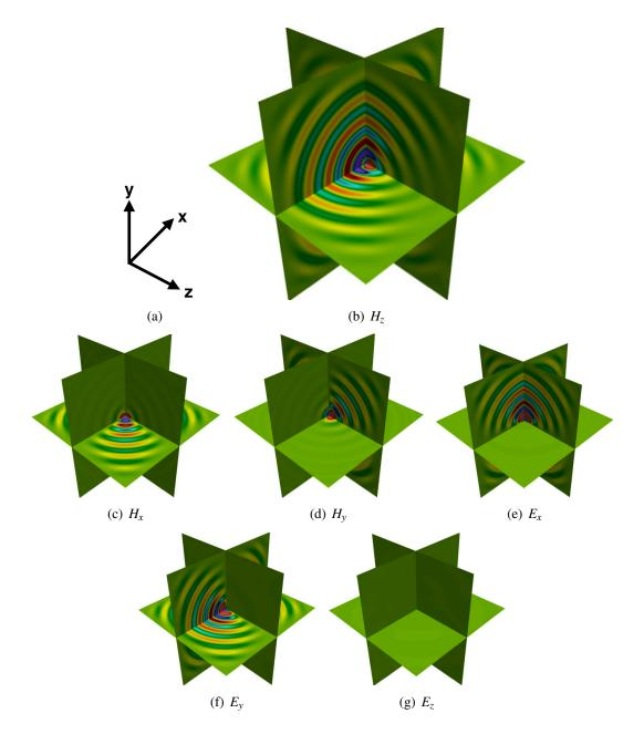
Fig. 10.1 (a) Axes of all plots are shown in this figure, (b)  $H_z$ , (c)  $H_x$ , (d)  $H_y$ , (e)  $E_x$ , (f)  $E_y$  and (g)  $E_z$  field distribution in space after 1000 time steps for a  $H_z$  point source at the middle of the computational domain.
