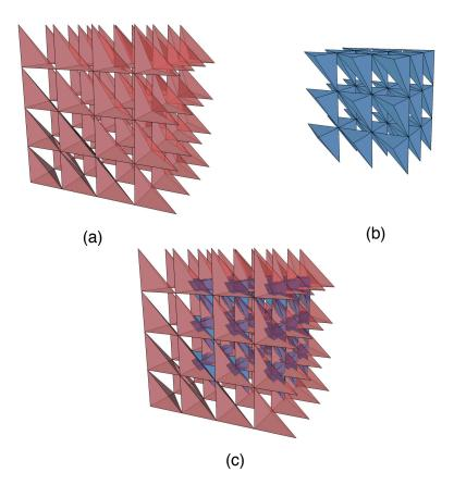
Fig. 8.2 (a)  $4 \times 4 \times 4$  main mesh generated by using the basic element of Fig. 8.1, (b) the  $3 \times 3 \times 3$  auxiliary mesh generated using the centroid of the main mesh elements in Fig. 8.2(a), (c) both meshes together
