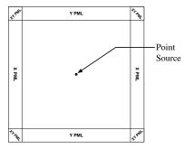
(a) Computational domain with a point source at the center and PML boundaries near the boundary of the domain
