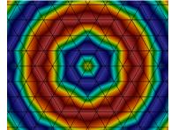
(g) Magnified view of the central region with mesh overlay of the field shown in Fig. 11.5f
