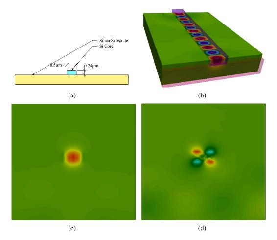
Fig. 10.3 (a) Cross section of the nanowire, (b) Propagation of  $H_y$  field inside the guide, (c) Mode profile of the dominant  $H_y$  field, (d) Mode profile of the non-dominant  $H_x$  field.
