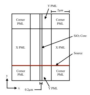
Fig. 6.3 Schematic diagram of the planner waveguide setup
