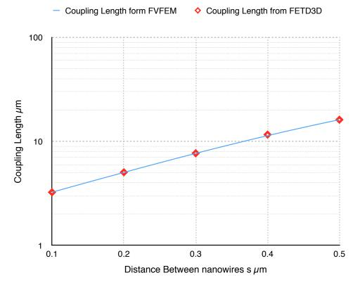
Fig. 10.9 Comparison of coupling length obtained from FVFEM and the proposed 3D FETD method
