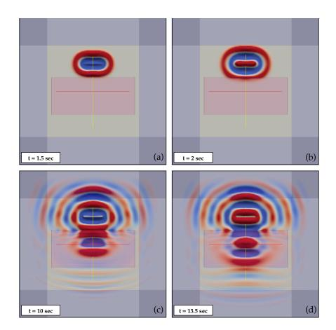
Fig. 6.6 (a) Line source radiating  $E_z$  field before incident on the DNG slab, (b) interaction of first half cycle with the DNG slab, (c) after a while when the wave start to propagation inside the DNG slab, (d) when the wave start to come out of the DNG slab on the other side
