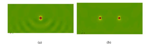
Fig. 10.5 (a)  $H_y$  field profile propagating in the nano input wire, (b)  $H_y$  field profile after splitting the input power into two at the output nanowires
