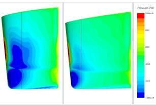
Figure 13 - Pressures on port side of Basic (left) and "Longback 1.4" rudders. The black lines indicate the widest point of the rudder
