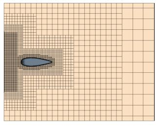
Figure 2 – Slice through a typical computational mesh
