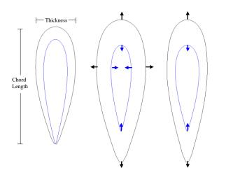
Figure 8 – Upper (black) and lower (blue) cross-sections of (l-r) Basic, Tapered 1.25 and Stretched 1.25 rudders. Arrows indicate the modification compared to the Basic rudder
