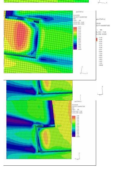
Figure 18. Starboard pintle velocity distribution during a 5 degree turn to port
