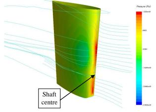
Figure 3 – Pressure contours on rudder with streamlines
