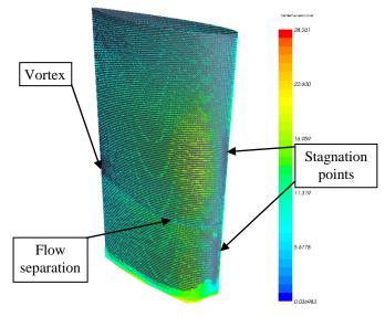
Figure 4 – Velocity vectors around the rudder
