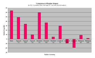
Figure 10 - Typical drags for rudder shapes
