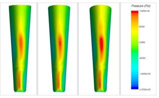
Figure 7 - Typical pressures on leading edge of rudder with hull angle (l-r)  $10^\circ, 5^\circ$  and  $0^\circ$
