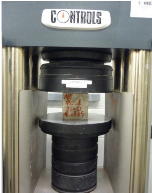
Figure 27. Cube compression test set up
