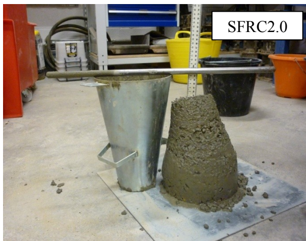
Figure 22. Slump measurement after mixing
