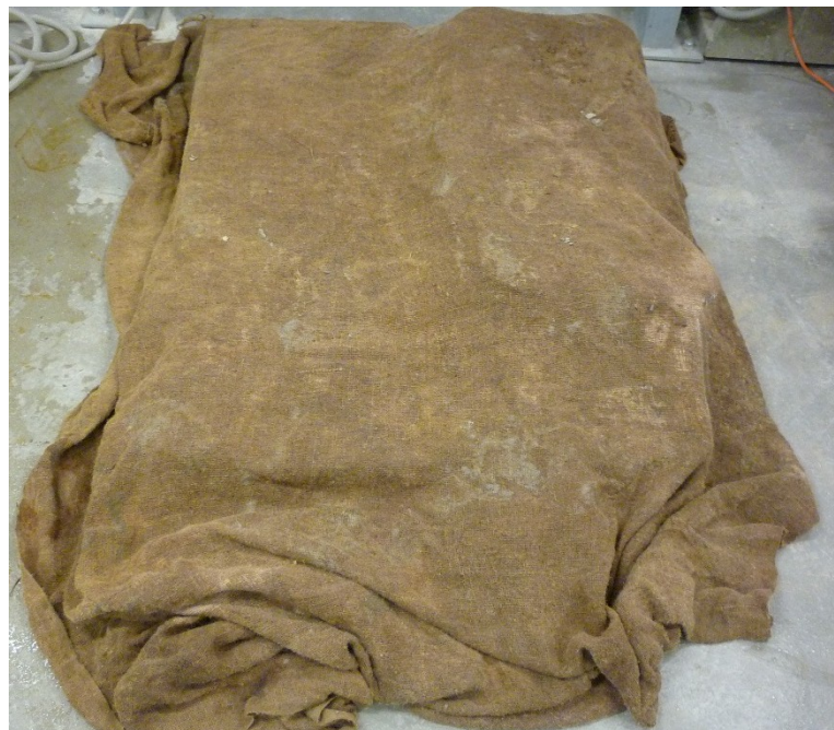
Figure 25. Covering of the specimen after casting with wet cloth
