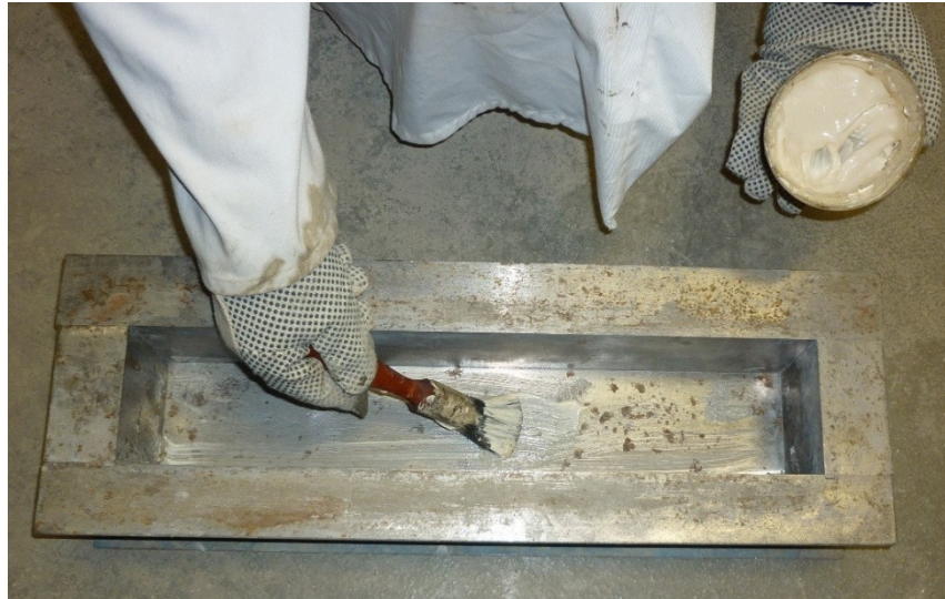
Figure 23. Covering inside the moulds with specific oil
