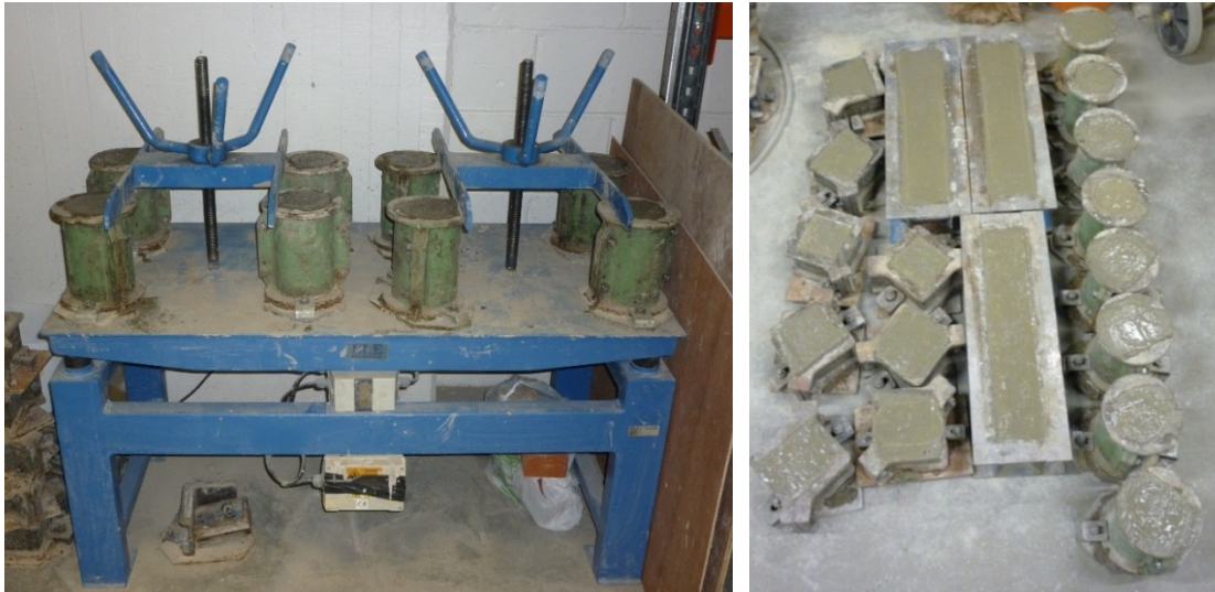
Figure 24. (a) sample moulds on shaking table, (b) Concrete moulds
