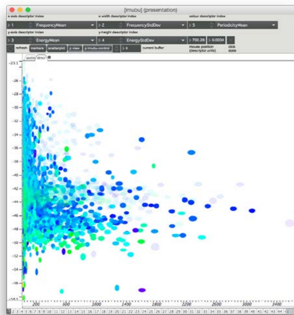
Figure 4: iMuBu scatterplot showing a corpus with some sound files (and their markers) disabled (transparent).
