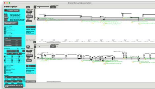
Figure 5: Transcription subpatch showing markers displayed in bach.roll and bach.score with slots for metadata.
