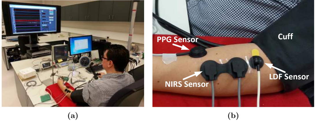
Figure 9.1: Measurement system set-up (a) and placement of PPG, NIRS, and LDF sensors on the forearm (b).
