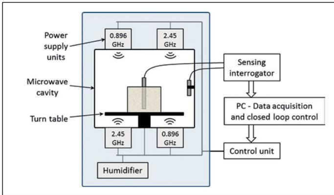
**Figure 2: Schematic of smart microwave oven system.**
