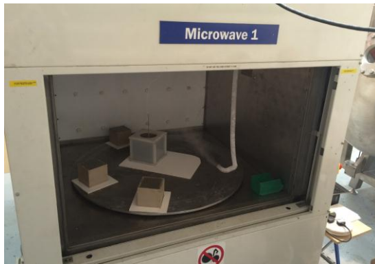
Fig. 8 Scaled-up trial of microwave-cured concrete
