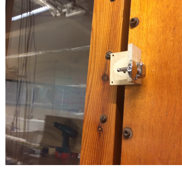
Figure 5: Mechanism to tighten the string upstream of the model
