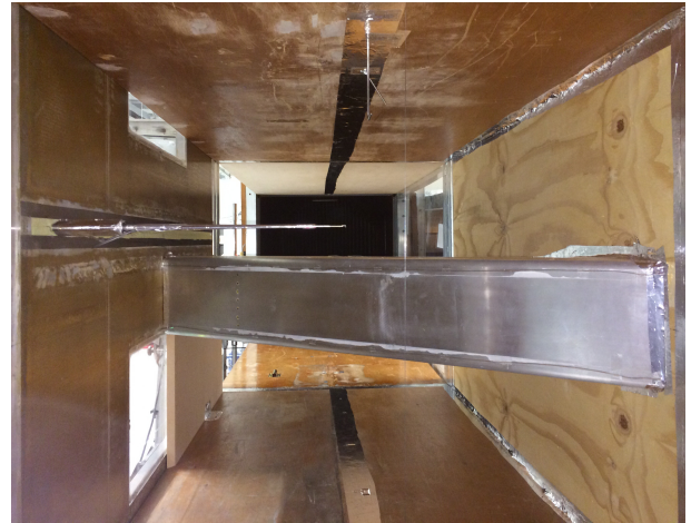
Figure 3: Blunt leading-edge wing mounted in the wind tunnel
