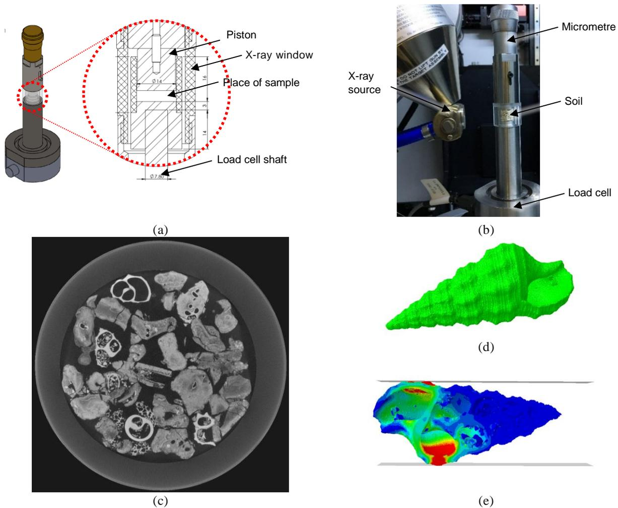
**Figure 1:** a) Schematics of the loading apparatus; b) x-ray source gun and soil sample; c) slice through the 3D image of the dry coarse sample; d) 3D model of a single grain; e) intra-granular stress distribution for a single grain compressed between two flat platens (cut view).
