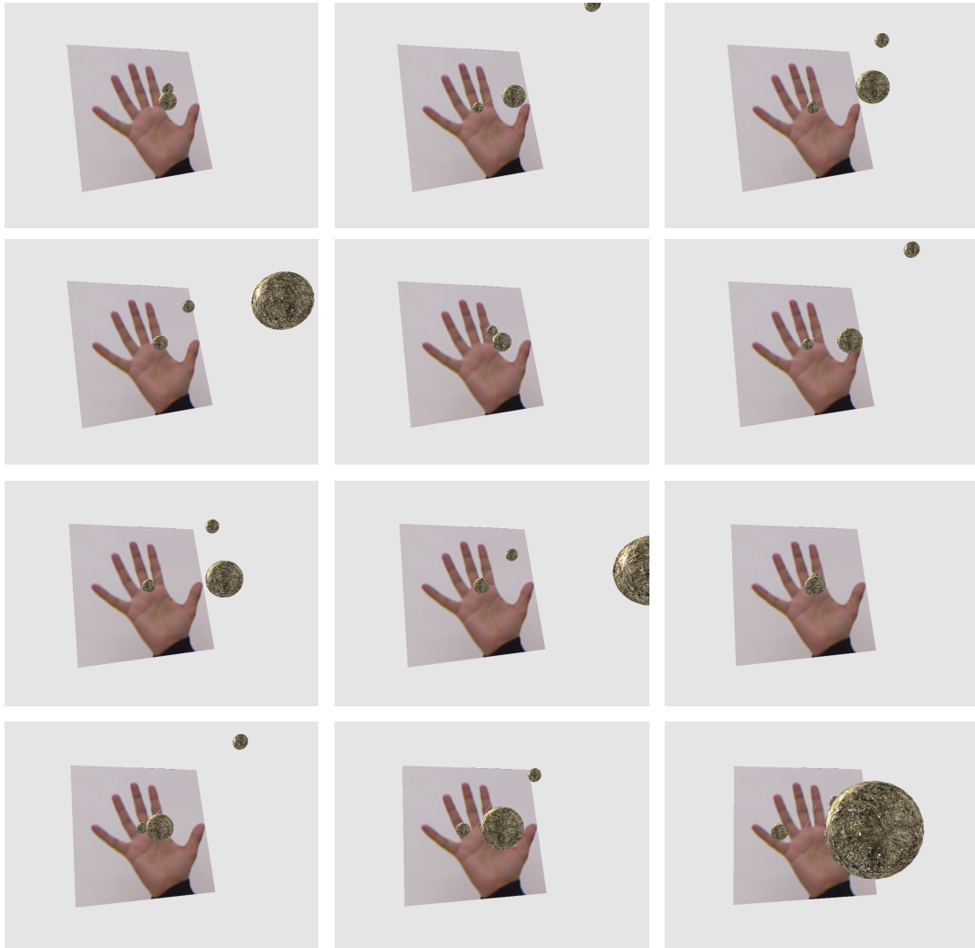
Fig. 4.11 Application of the proposed approach to an Augmented Reality game. The objective of the game is to deflect the incoming balls to target directions using the orientation of the hand. The sequence of hand orientations starts from the top left and ends at the bottom right image.
