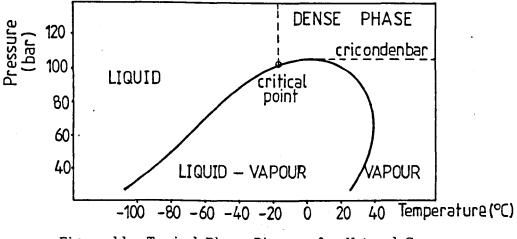
Figure l.l. Typical Phase Diagram for Natural Gas
