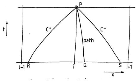
Figure 4.3. Effect of Flow Reversal on the Characteristics.
