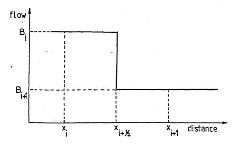
Figure 3.11. Discontinuity between two half sections
