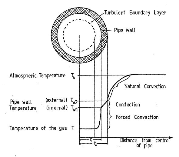
Figure 2.4. Heat Transfer into the pipe.
