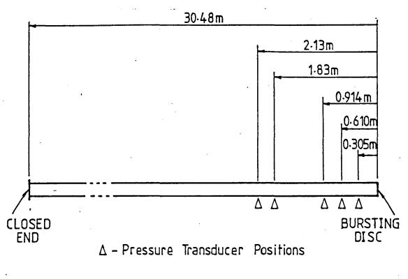
Diameter of Shock Tube = 0.0603m
