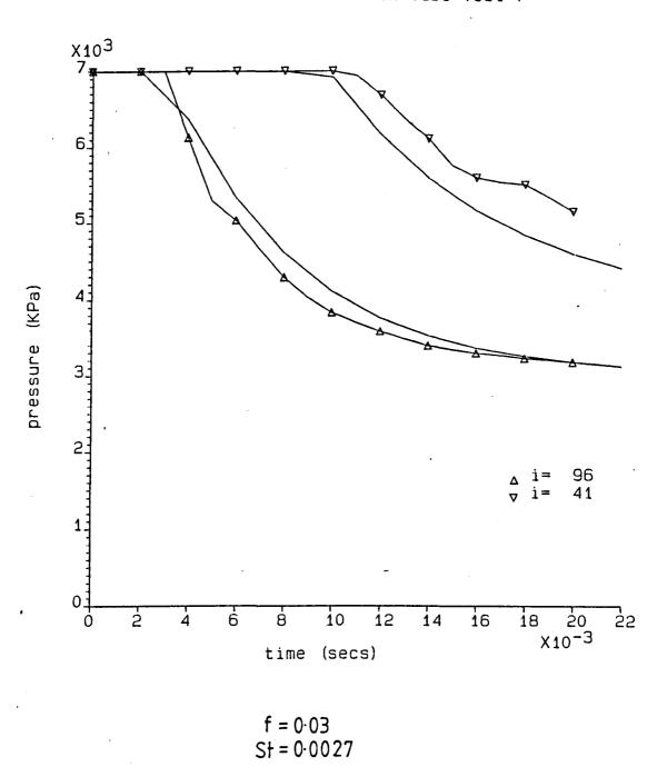
Figure 7.14. P x t Graph for British Gas Shock Tube Test 7
