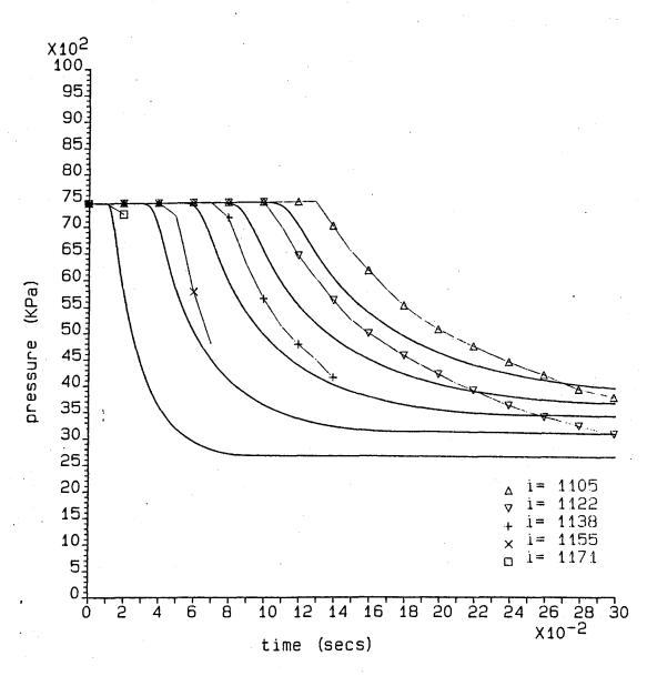
Figure 7.25. P x t Graph for Foothills Test Results NABTF5 (West)
