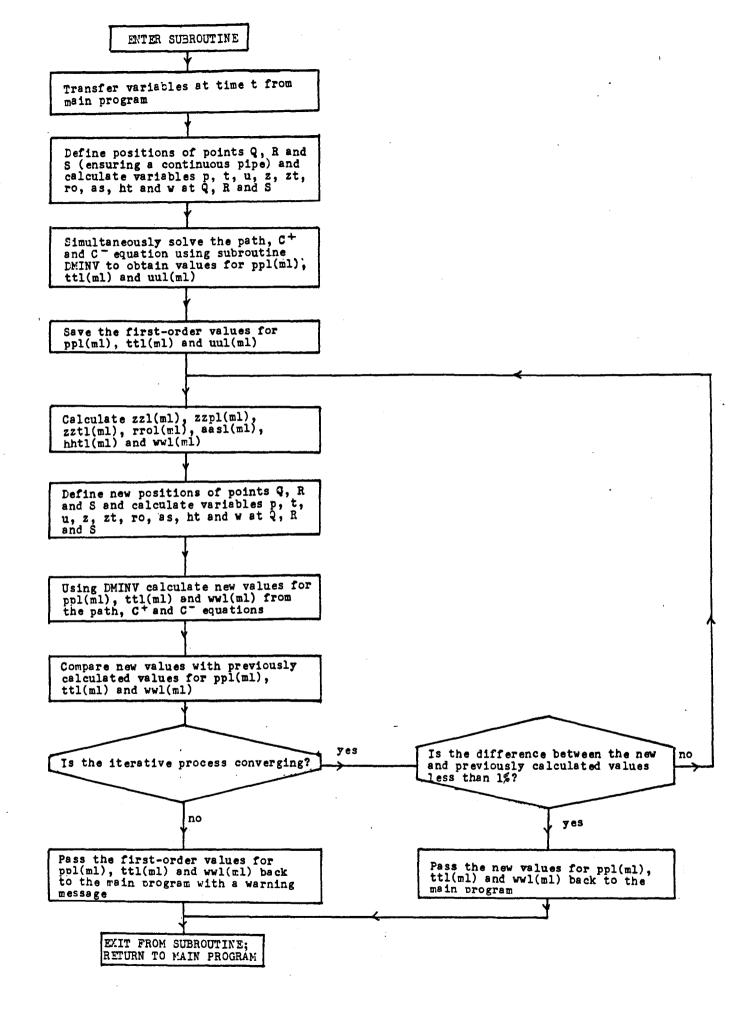
Figure 5.8(a) Flow Diagram for BREAK1
