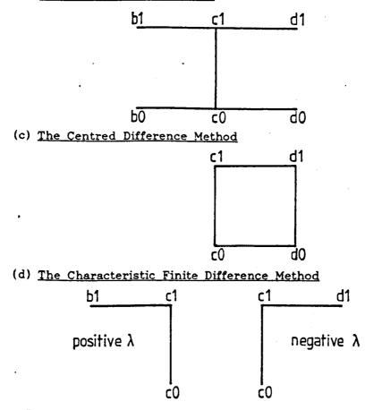
Figure 3.8. Grid points used in various Finite Difference Methods
