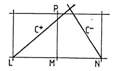
Varying wavespeed flow - In order to satisfy the stability criteria in the high wavespeed region interpolation errors may be incurred in the low wavespeed region
