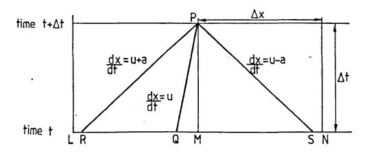
Figure 3.4. Characteristics for three dependent variables on a rectangular grid
