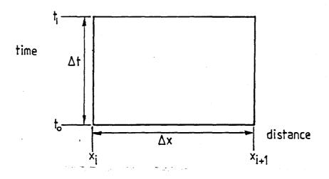
Figure 3.10. Elemental section for flux difference splitting
