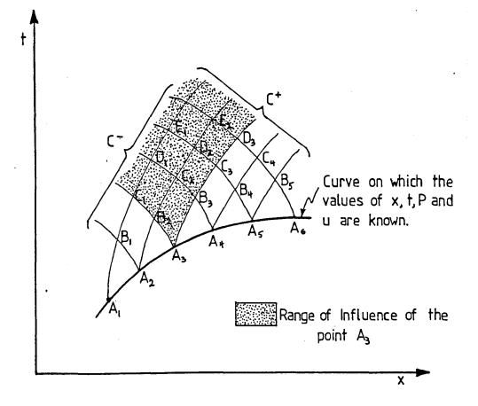
Figure 3.1 Two-dimensional natural grid of characteristics
