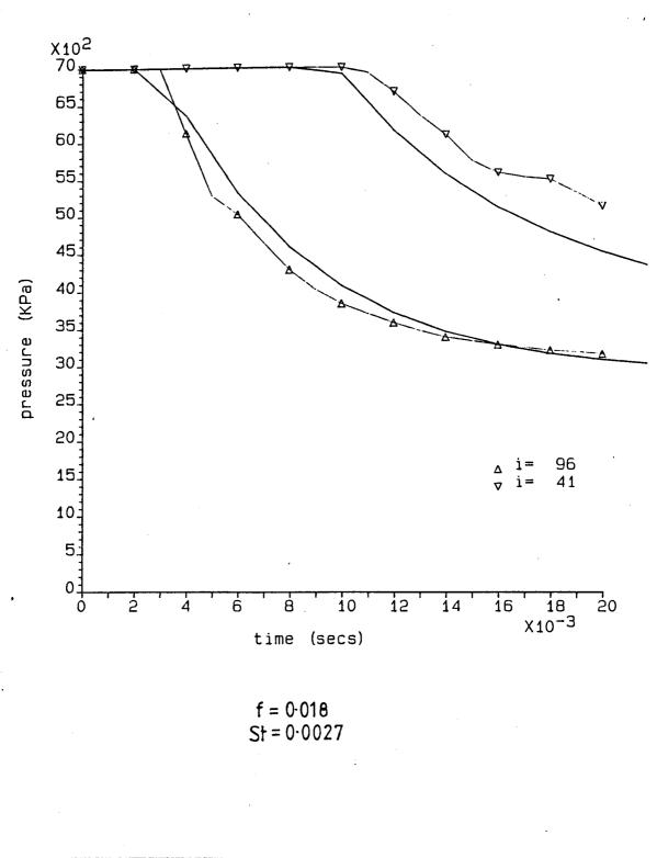
Figure 7.8. P x t Graph for British Gas Shock Tube Test 7
