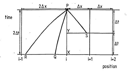
Figure 4.4. Grid point linking two different grid sizes
