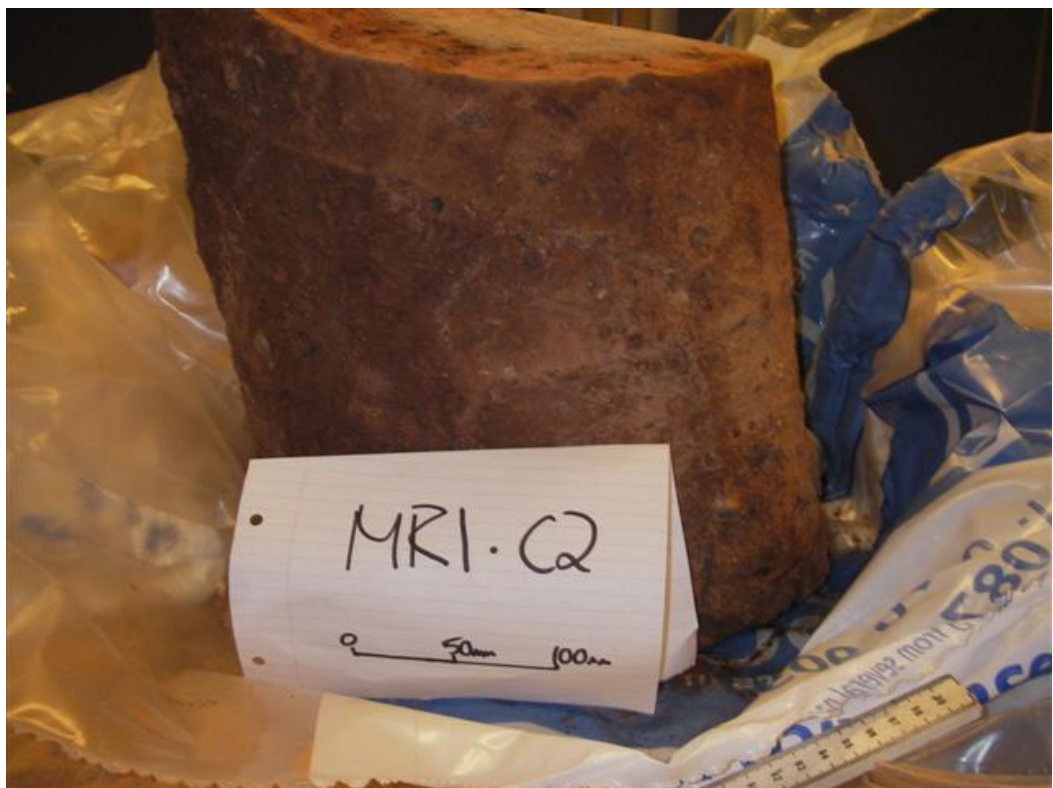
Figure 4.10 The section from pile MR1 495-819mm below ground level
