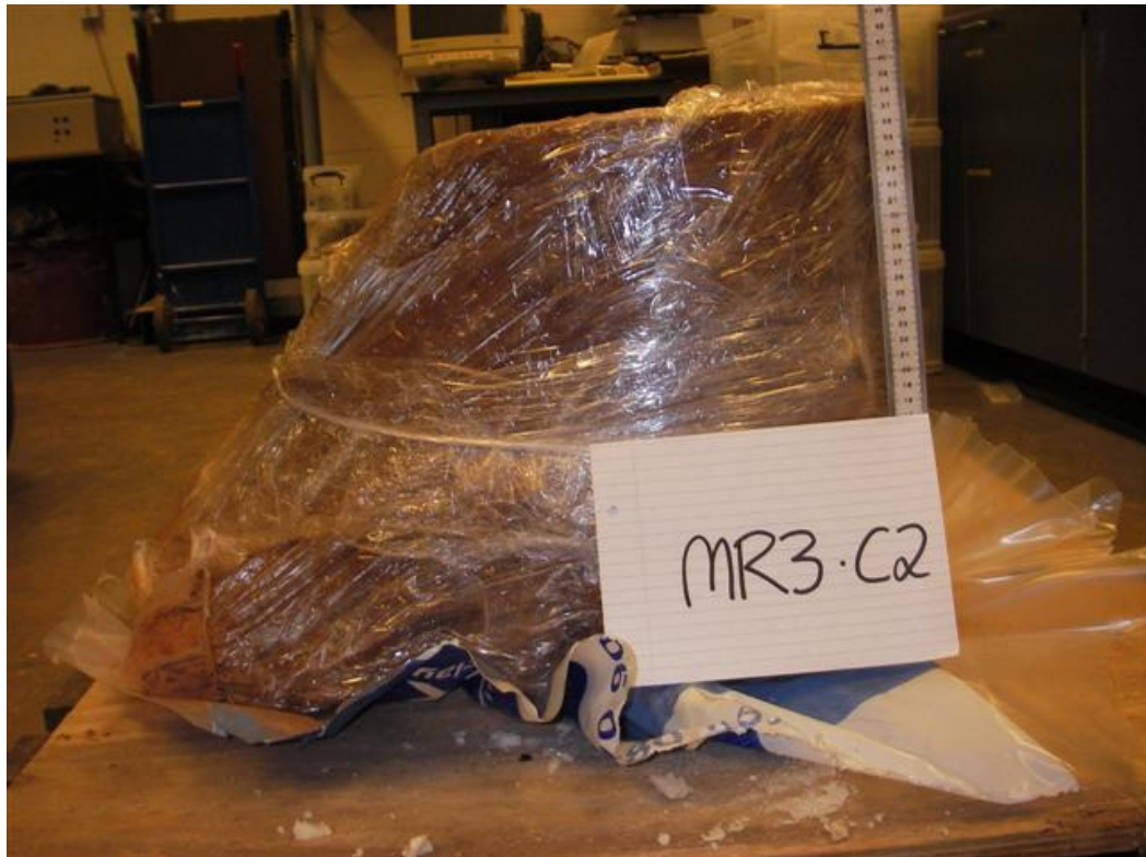
Figure 4.27 The second section from pile MR3 510-860mm below ground level
