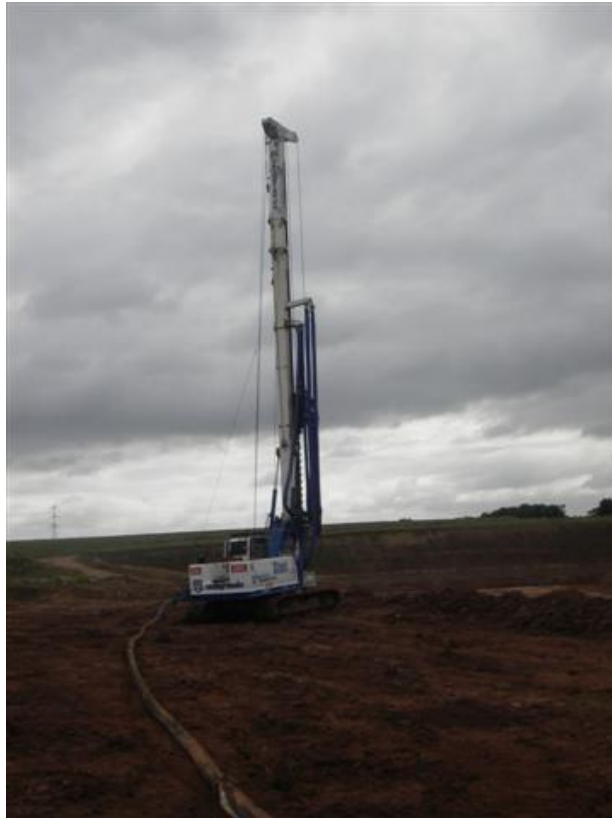
Figure 3.4 The rig used to install test piles
