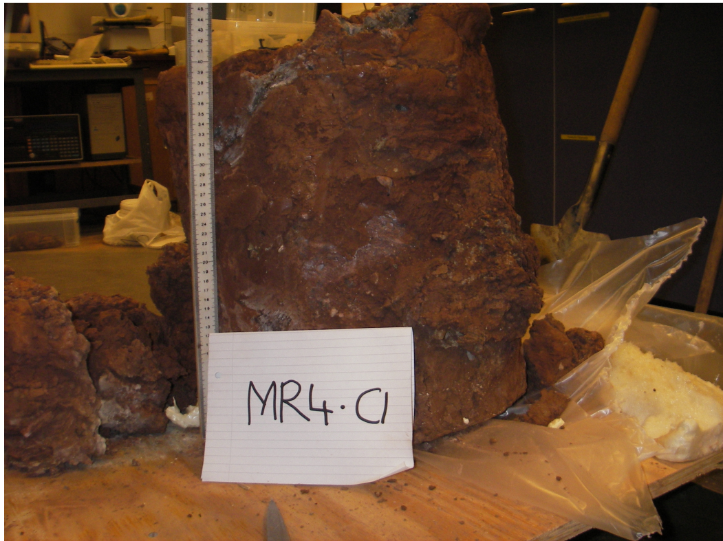
Figure 4.38 The first section taken from pile MR4 0-451mm below ground level
