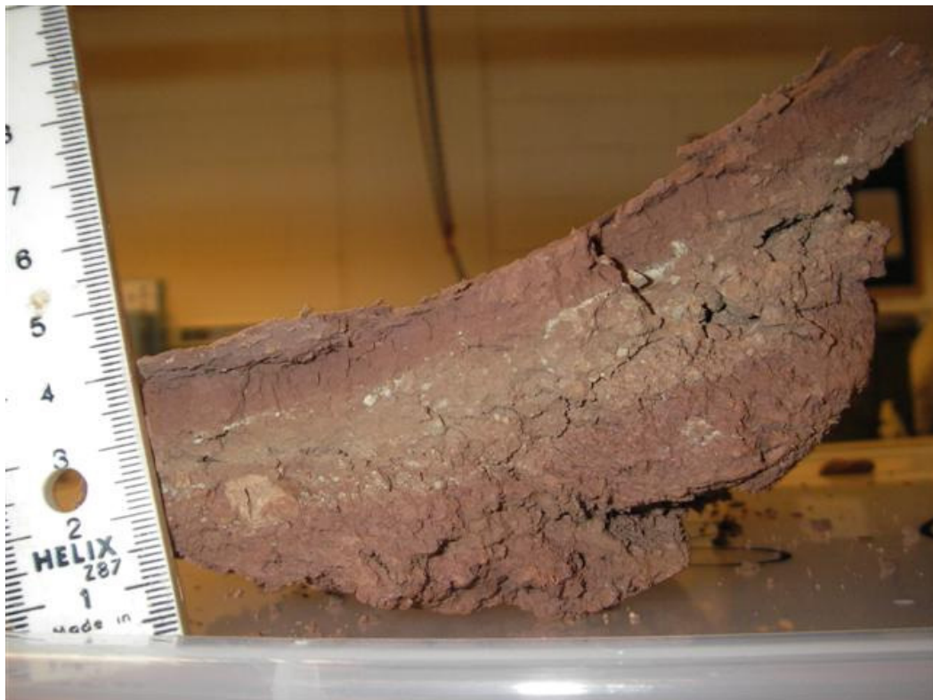
Figure 4.33 Zoning of remoulding with the soil surrounding pile MR3 860-1210mm below ground level. Then soils is viewed from above, and the pile would have been at the top of this picture
