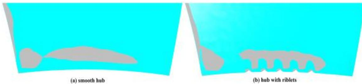
Figure (12): Stream-wise vortex structure over hub surface
