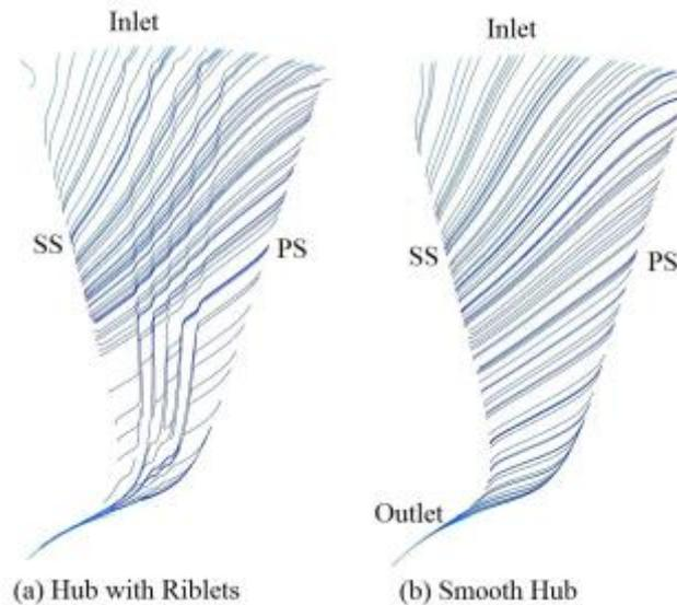
Figure (11): Limiting streamlines at the rotor hub
