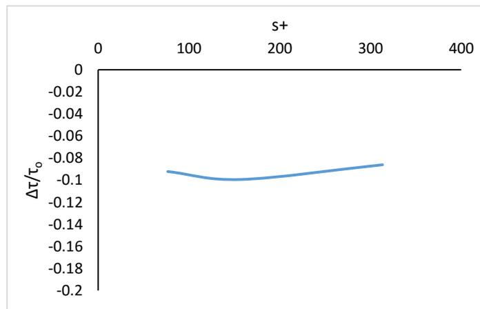
Figure (17): drag reduction for different riblets spacing
