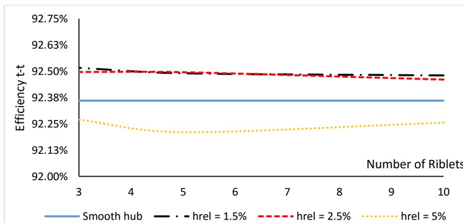
Figure (20): Turbine performance for different riblets geometry
