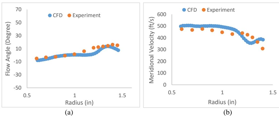
Figure (6): Spanwise distribution of (a) flow angle (b) meridional velocity at rotor discharge
