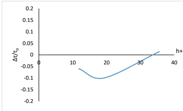
Figure (18): drag reduction for different riblets spacing
