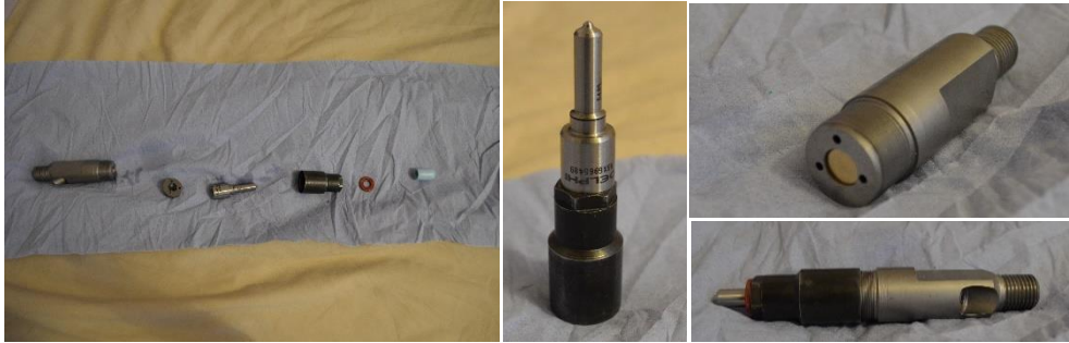
Figure 70 Needleless 0.213 mm hole diameter, low carbon Steel Delphi HB X 6965489
