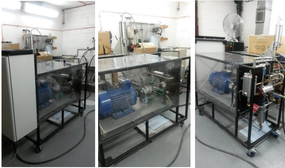
Figure B 2 - 1 Continuous Flow Sustained Hydrodynamic Cavitation Rig
