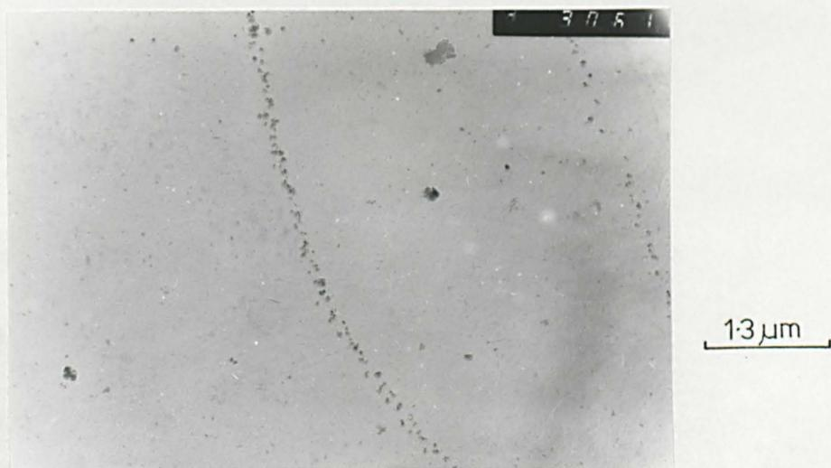
Fig.10.20 AlN precipitation in C-Mn-Al-Ca steel tested at 850°C using a strain rate of  $3 \times 10^{-3} \text{ s}^{-1}$ .
