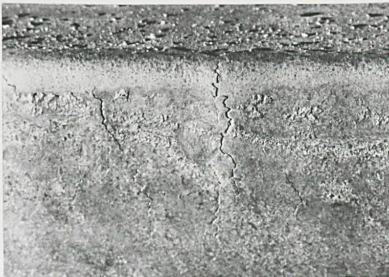
Fig.2.1 Cold machine scarfed slab showing transverse cracking.
