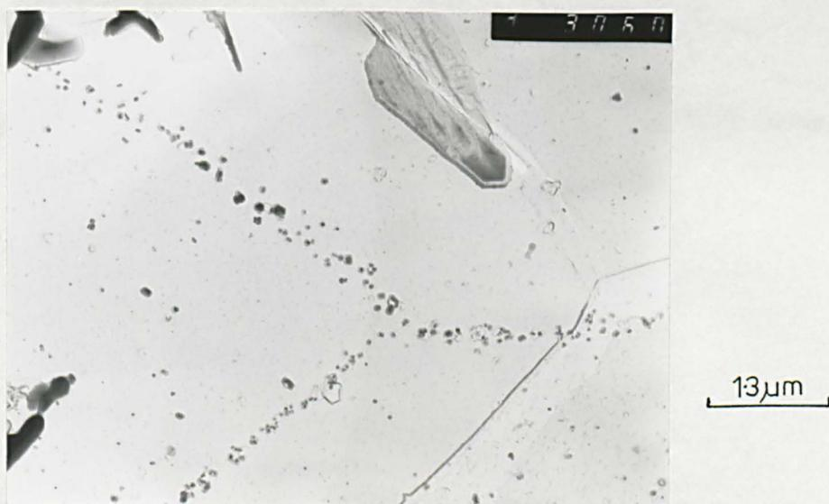
Fig.10.21 AlN precipitation in C-Mn-Al-Ca steel tested at 1050°C using a strain rate of  $3 \times 10^{-3} \text{ s}^{-1}$ .
