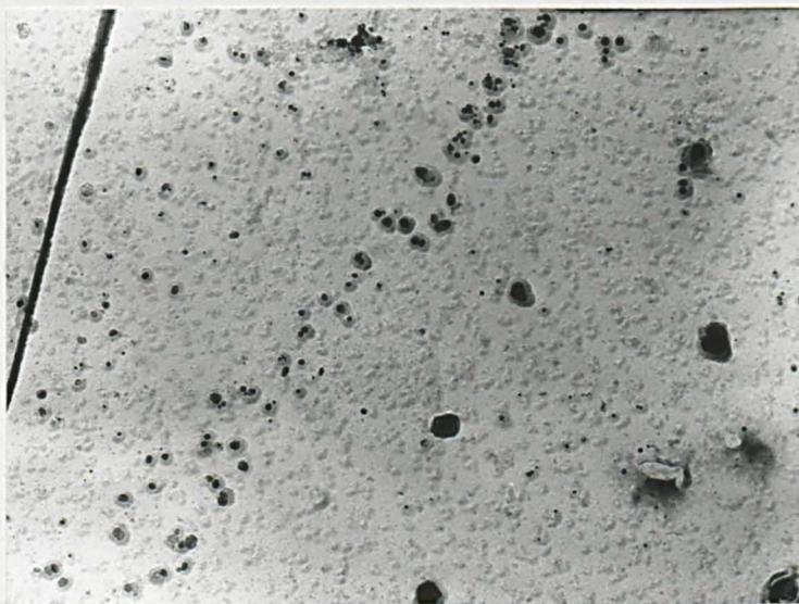
Fig.10.26 Precipitation in C-Mn-Nb-Al steel tested at 850°C using a strain rate of  $3 \times 10^{-3} \text{ s}^{-1}$
