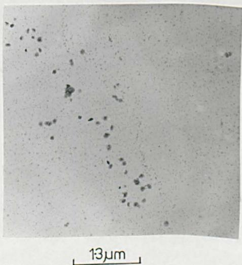
**Fig. 8.10** Precipitation in continuously cast C-Mn-Nb-Al slab a) surface
