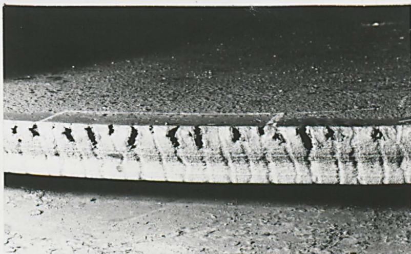
Fig.2.2 Slab which had been partially rolled showing severe transverse edge cracking.
