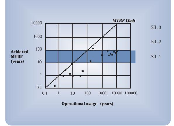
COTS software data from nuclear, chemical and aerospace (control and protection) industries. Claimed MTBF is limited to the total usage time. Some systems exhibit growth rates 100 times less than the best case.
