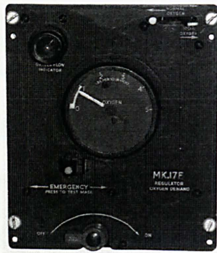
Figure 3.2 Front panel view of Mk17F pressure-demand breathing gas regulator
