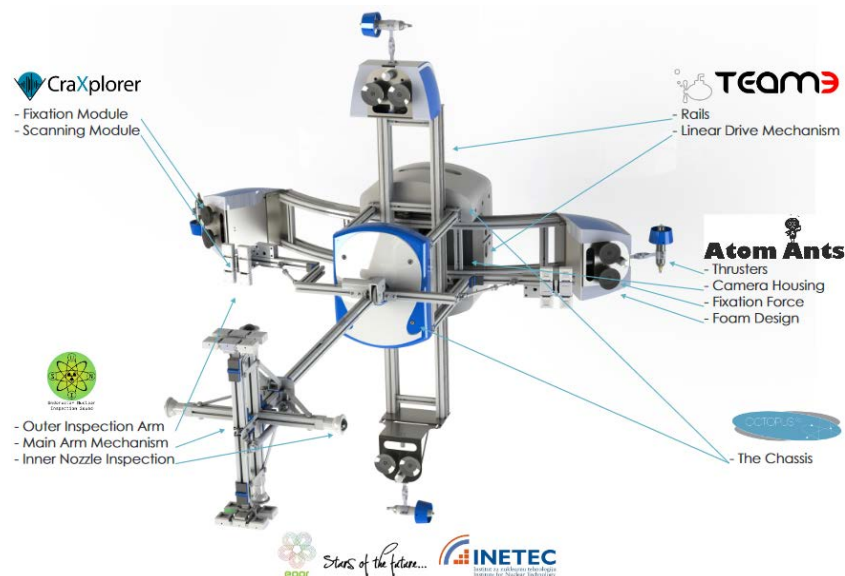
Figure 1. Remotely operated device for inspecting welds in nuclear reactors, Zagreb 2015
