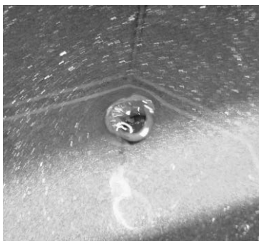
Figure 3: Oblique view on the water surface showing the rotation of the ambient fluid (4 min after release of the ice-particle on the surface). The period of one revolution of the ice-particle is T = 3 \text{ s} .
