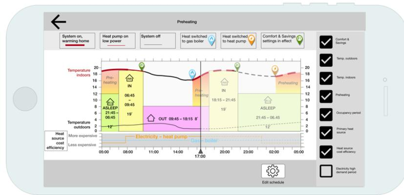
Figure 4. Detailed wireframe for graphical explanation of pre-heating.
