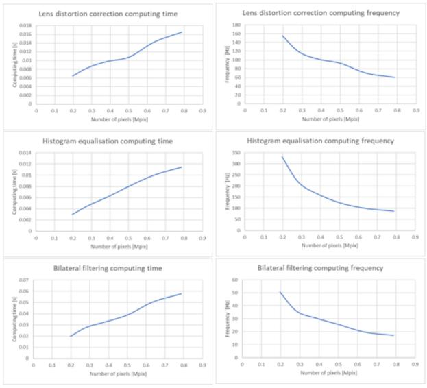
Fig. 4. Computing times for image pre-processing algorithms.
