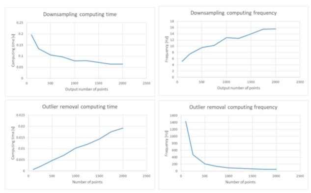
Fig. 3. Computing times for point cloud pre-processing algorithms.
