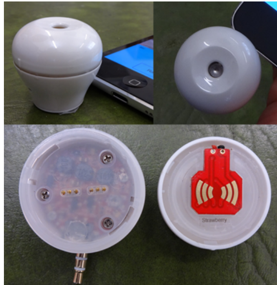
Figure 4.7: Scentee consists of a motor unit and a tank for liquid odorants.
