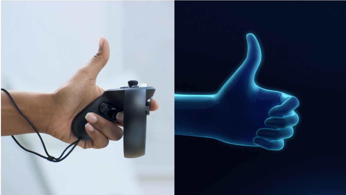
Figure 5.3: Oculus Touch hand tracking in real world (left) and virtual representation (right) (Touziet, 2016).
