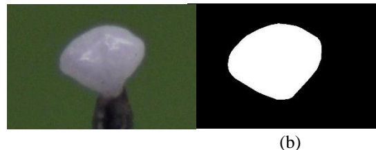
Figure 1 (a) 2D projection of a silica sand grain showing the green photography background, pedestal, and sand grain, (b) Binarised 2D projection.
