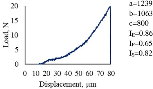
Figure 6 Load-Displacement curve of LB2
