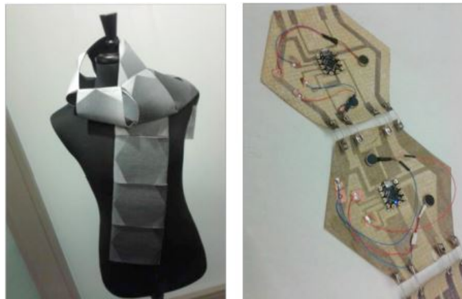
Figure 12 Scarf form factor and modular soft circuits on Microsoft Research's SWARM Prototype
