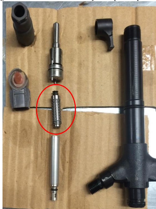
Figure 3.1.3 TOYOTA injector piezo spill valve
