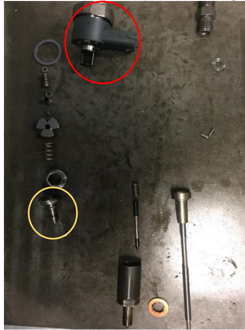
Figure 3.1.2 VAUXHALL injector solenoid spill valve
