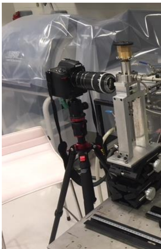
Figure 7.1.1 Nikon NIKKOR D7000 setup for photographic imaging of fluorescence phenomenon
