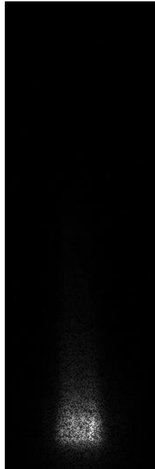
Figure 7.2.2 Fluorescent diesel flow at 200bar upstream pressure image taken at \frac{1}{\text{frame}} s shutter speed using Photron APX-RS high speed camera
