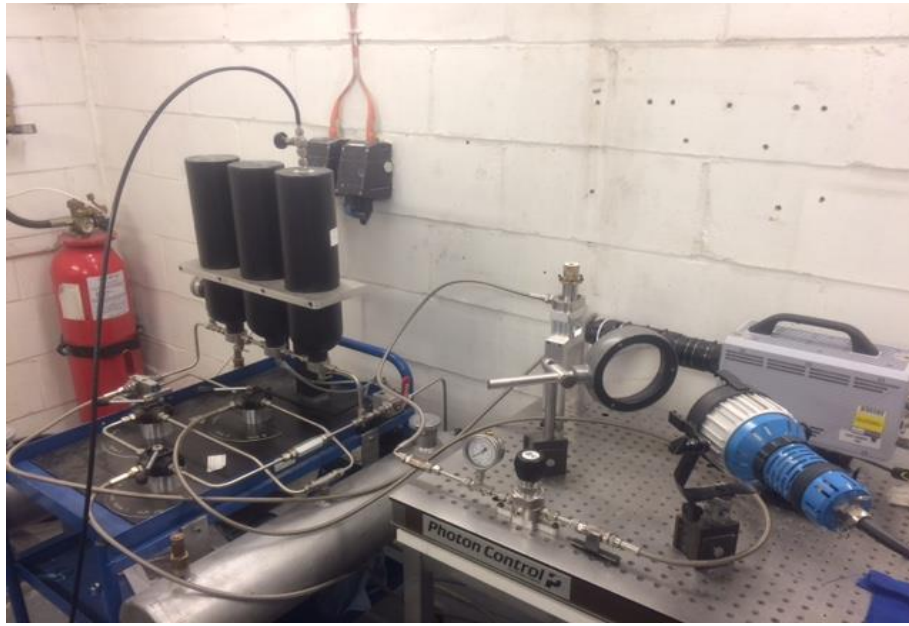
Figure 3.3.2 Experimental setup of low pressure characterisation test
