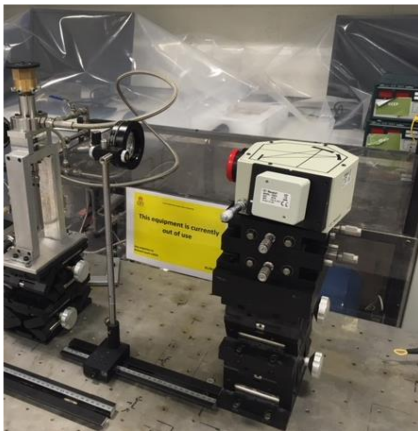
Figure 7.1.3 Oriel 77400 MS125 spectrometer setup for spectrum analysis of fluorescence phenomenon
