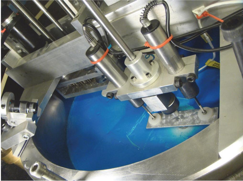
Figure 4.28 Top tube mounted to soil container with instrumentation attached.
