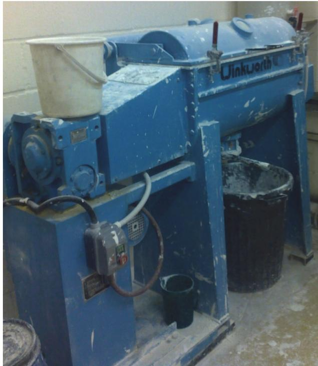
Figure 4.20 Photograph of industrial ribbon blade mixer.
