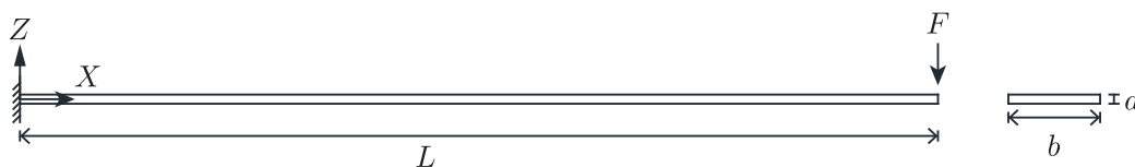
Figure 3.8: Cantilever subjected to end point load.
