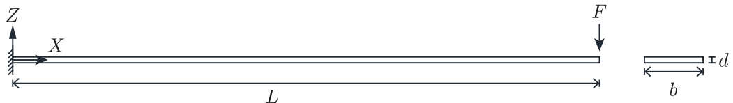
Figure 4.3: Cantilever subjected to an end point load.
