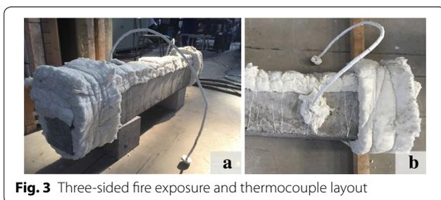
**Fig. 3** Three-sided fire exposure and thermocouple layout
