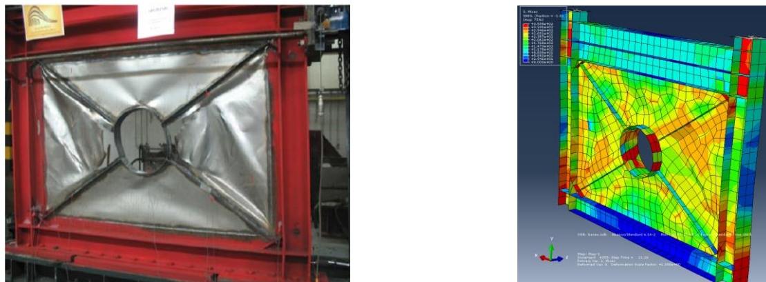
Fig. 5. The deformed shape of the specimen from the experimental test (Alavi and Nateghi [Error! Reference source not found.20]) and numerical model at 4.4% drift.
