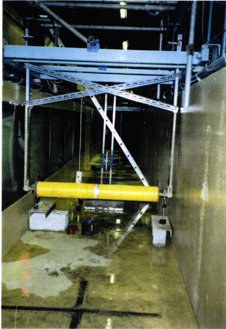
Fig: 7.1 (a) Carriage, test cylinder and related instrumentation
