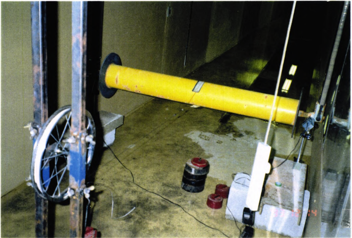
Fig: 7.1 (b) Carriage, test cylinder and related instrumentation
