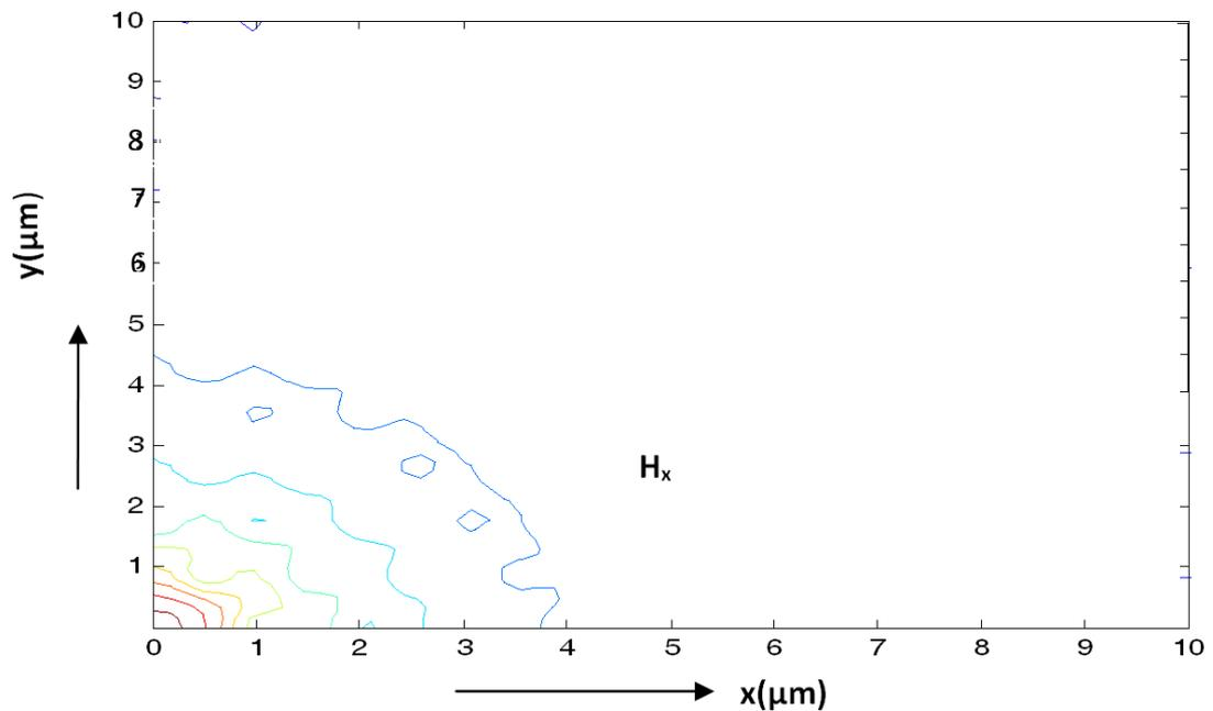
Fig. 6. 7:  $H_x$  field profile of the  $H_{11}^x$  mode for  $N = 7$ ,  $\Lambda = 1.0$ ,  $d/\Lambda = 0.4$ , and  $d_7/\Lambda=0.8$ .
