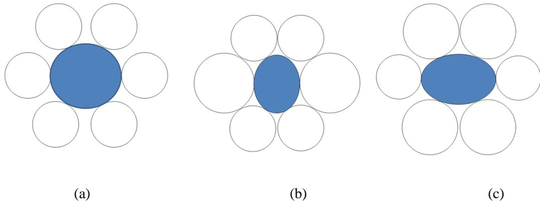
Fig. 5. 2: The core and the first ring of air-holes in a PCF (a) with all the air-holes of the same diameter thus the core is circular (b) two larger air-holes on the side of the core making the core elliptical, height  $>$  width (c) two larger air-holes above the core and two larger air-holes below the core makes the core elliptical, width  $>$  height.
