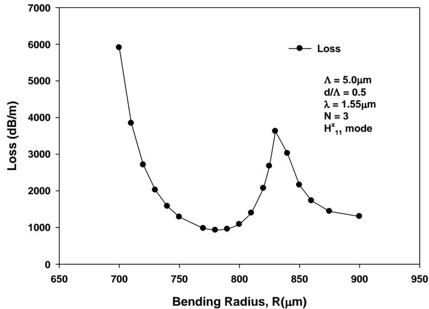
Fig. 4. 18: The variation of bending loss against bending radius, R, for values of R between 700μm to 900μm, when  $\Lambda = 5.0\mu\text{m}$ ,  $d/\Lambda = 0.5$ .
