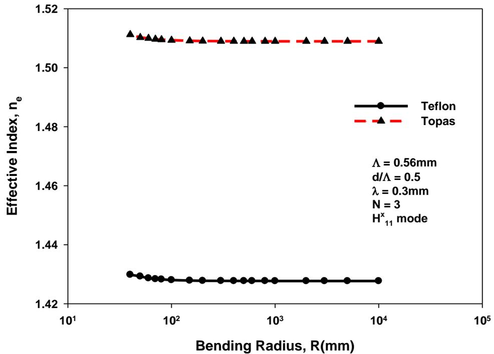
Fig. 7. 6: Graph comparing effective index in Teflon and TOPAS with respect to bending radius.
