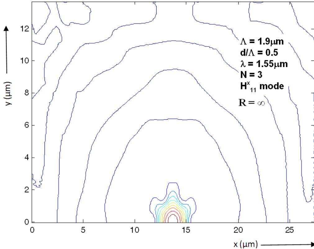
Fig. 4. 10:  $H_x$  field contours for the  $H_x^{11}$  mode  $R = \infty$ ,  $\Lambda = 1.9\mu\text{m}$ ,  $d/\Lambda = 0.5$ .
