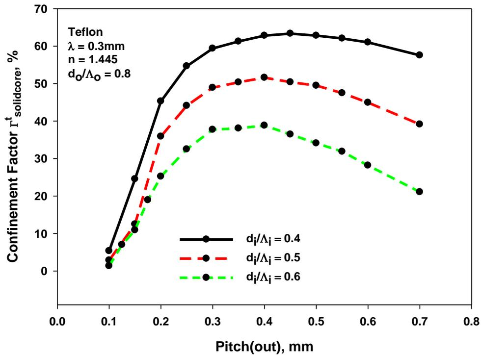
Fig. 7. 32: Variation of the confinement factor in the core air-holes,  $\Gamma_{\text{solidclad}}^{\text{a}}$ , with the outer pitch  $\Lambda_o$  for  $d_o/\Lambda_o = 0.8$  but with different  $d_i/\Lambda_i$  values.
