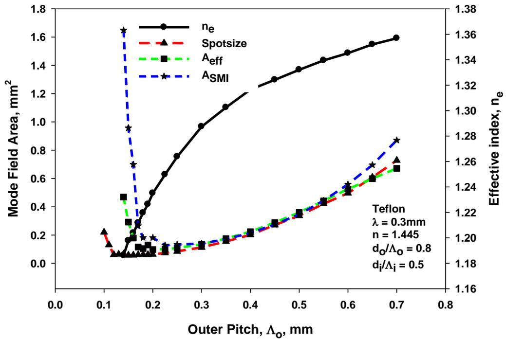
Fig. 7. 25: Variations of the mode field areas and effective index with the pitch,  $\Lambda_o$  for  $d_o/\Lambda_o = 0.8$  and  $d_i/\Lambda_i = 0.5$  for  $H_{x11}$  Mode.
