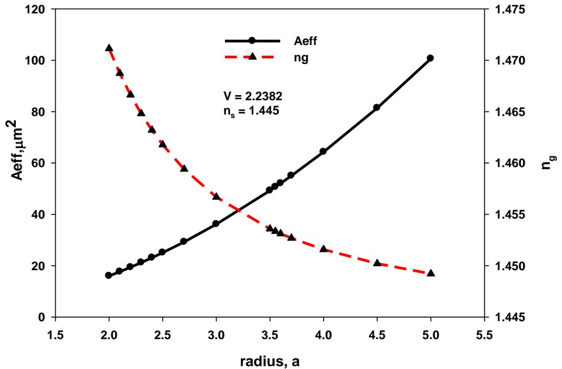
Fig. 6. 15: Variation of  $A_{\text{eff}}$  and core refractive index difference,  $n_g$  of a SMF against fibre radius,  $a$ .
