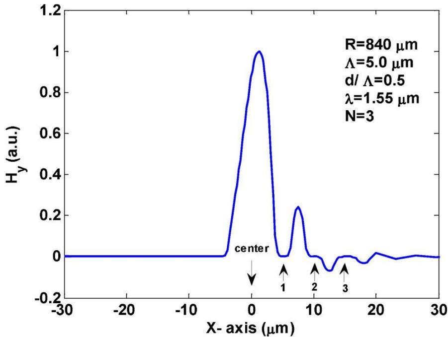
Fig. 4. 23: Variation of the  $H_y$  field along the x-axis for  $R = 840\mu\text{m}$ ,  $\Lambda = 5.0\mu\text{m}$ ,  $d/\Lambda = 0.5$ .
