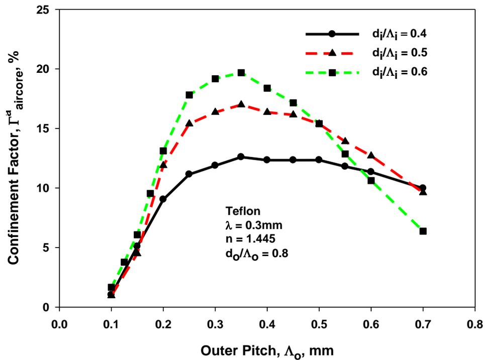
Fig. 7. 30: Variation of the confinement factor in the core air-holes,  $\Gamma^a_{\text{aircore}}$ , with the outer pitch  $\Lambda_o$  for  $d_o/\Lambda_o = 0.8$  but with different  $d_i/\Lambda_i$  values.
