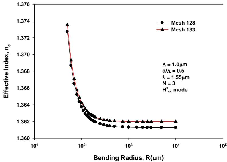
Fig. 4. 2: The variation of effective index of  $H_{11}^x$  mode with bending radius for mesh divisions 128 x 65 and mesh 133 x 70.
