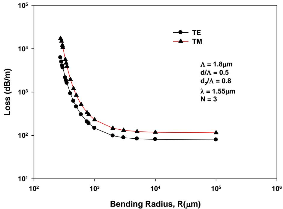
Fig. 5. 12: Variation of loss with the bending radius,  $R$  for  $\Lambda = 1.8\mu\text{m}$ ,  $d/\Lambda = 0.5$ ,  $d_2/\Lambda = 0.8$  for both quasi-TE and quasi-TM modes.
