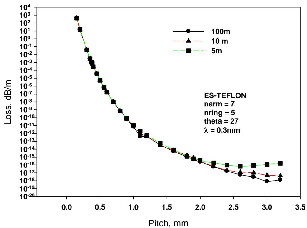
Fig. 7. 21: Graph comparing loss (without material loss) of Equiangular spiral Teflon with respect to pitch for bending radius of 5,000mm, 10,000mm and infinity.
