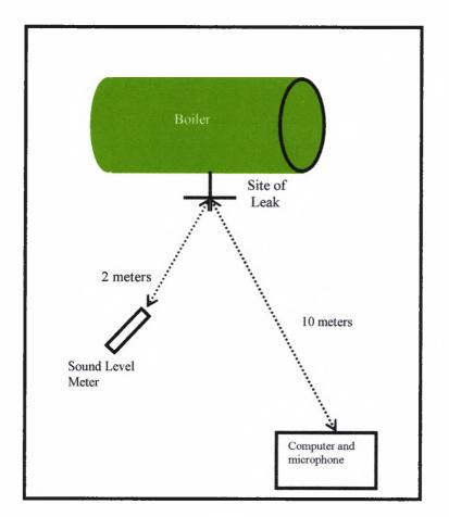
Figure 6.8 Experimental set up
