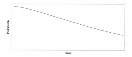
Figure 4.3 Pressuriser change for rod drop at 30 % power
