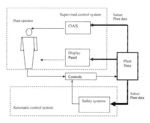
Figure 3.4 Plant Operation sub-systems
