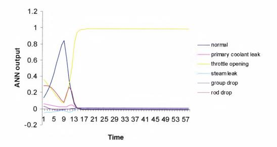
Figure 4.16 Throttle Opening Transient
