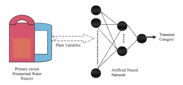
Figure 4.1 Classification of a transient based on feature set from a PWR
