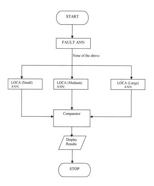
Figure 7.8 Flow diagram of LOCA Classification
