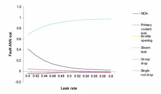
Figure 7.16 Fault ANN output for a range of downstream steam leaks
