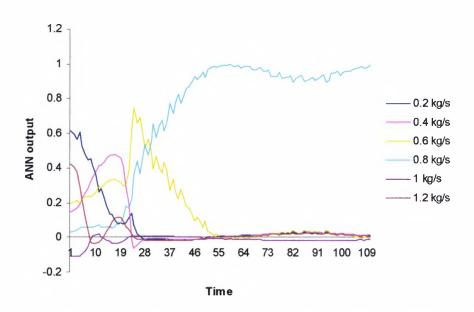
Figure 5.3 ANN output for a 0.8kg/s loss of coolant accident at 10% full power
