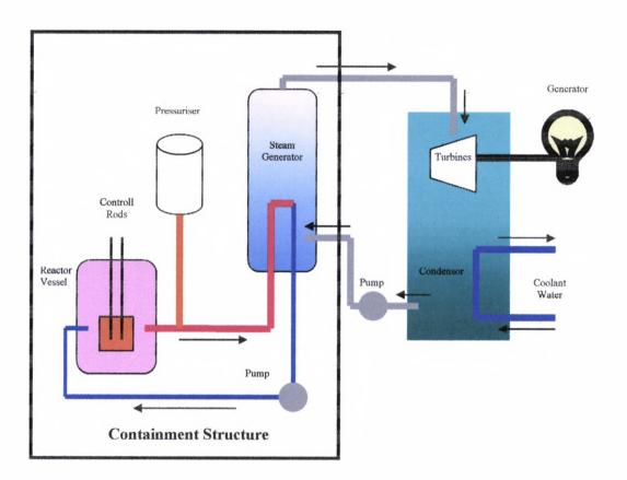
Figure 3.1 Schematic of a PWR
