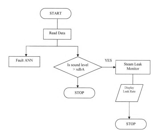
Figure 7.15 Implementation of Steam leak Monitor
