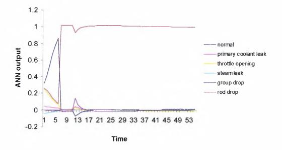
Figure 4.19 Single Rod Drop Transient
