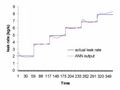
Figure 7.6 Estimation of large size leak rates
