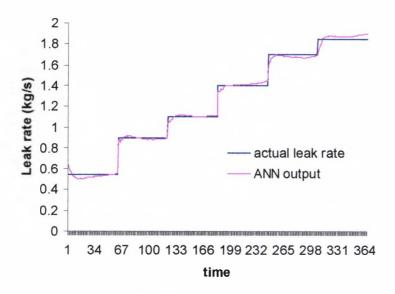
Figure 7.5 Estimation of medium size leak rates
