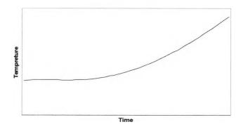
Figure 6.2 Temperature change for secondary circuit steam leak of 0.3 kg/s
