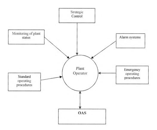
Figure 3.6 supervised control system with operator advisor
