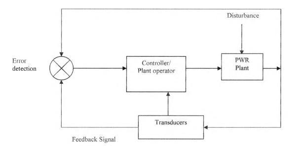
Figure 3.5 Block Diagram of a control system
