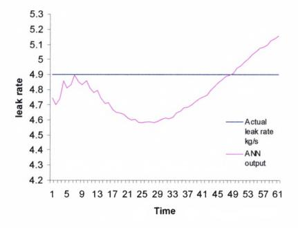
Figure 7.7 Estimation of a leak rate of 4.9 kg/s
