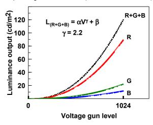
Fig. 3.3 The luminance output of the three phosphors of the SONY 500PS monitor are nonlinear functions of the applied voltage signal. The total luminance of the white light emitted by the combined signal of the three phosphors follows a power-law response to voltage whose exponent, known as gamma, has a typical value of 2.2. Data obtained using a LMT luminance meter (model 1003, www.lmt-berlin.de).
