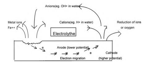
Figure A.2 Simple Corrosion Cell
