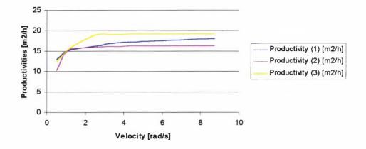
Figure 9.10 Productivity of MPIR with 2.3m Reach for Varying Velocity Profiles
