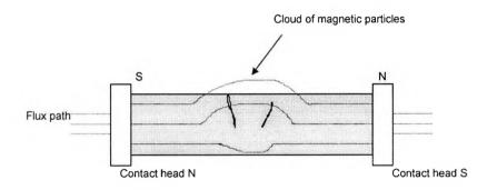
Figure 5.3 Test Piece in Magnetic Flow Detection
