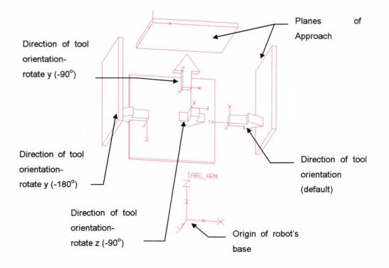
Figure 4.16 Schematic Idealisation of Tool Orientation
