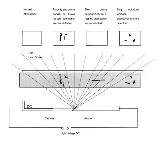
Figure 5.1 X-Radiography Testing (RT)
