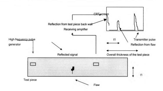
Figure 5.2 Ultrasonic Testing (UT)
