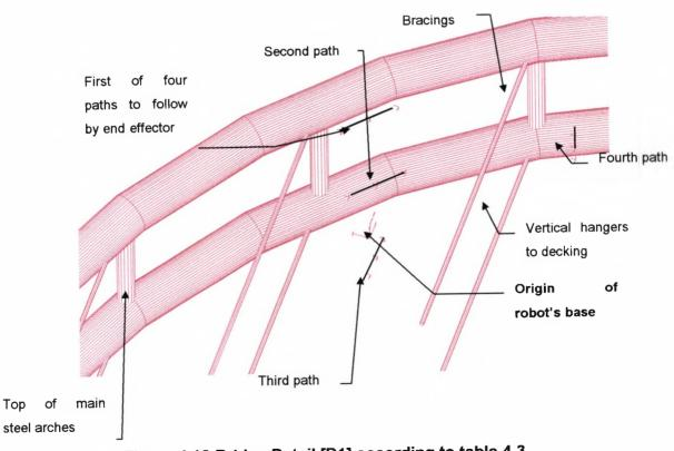
Figure 4.10 Bridge Detail [D1] according to table 4.3
