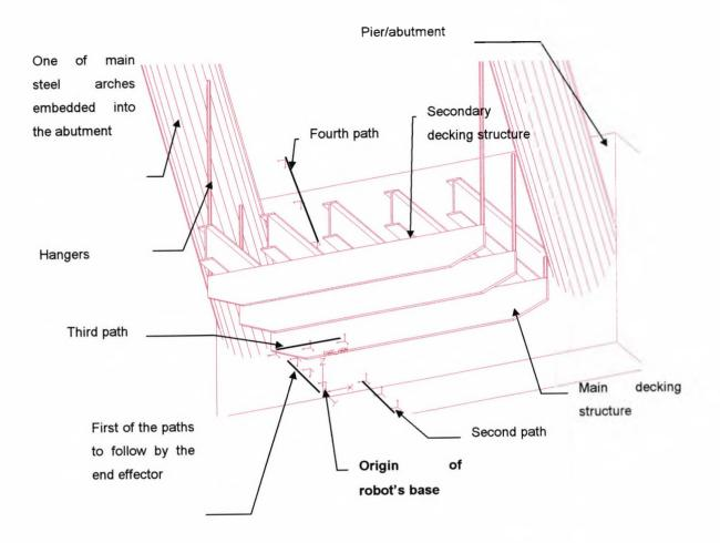
Figure 4.11 Bridge Detail [D2] according to Table 4.3
