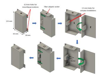
Fig. 3. Surface-mounted tilt sensor assembly procedure.
