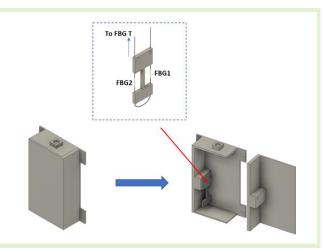
inclination changes during the test period. This compact, robust, and easy-to-install tilt sensor has excellent potential for various geotechnical applications, mainly in landslide detections, ground movement, and engineered slope monitoring.
