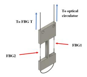
Fig. 2. FBG installation to the actuator.
