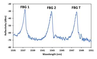
Fig. 7. Initial wavelength spectrum of the device at a  $0^{\circ}$  of tilt angle shows three reflective peaks of FBG1, FBG2, and FBGT.
