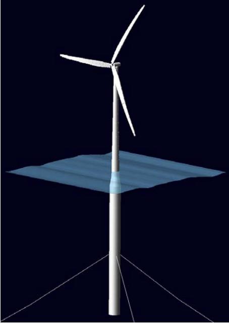
Fig. 1. 5MW NREL with OC3-Hywind spar buoy platform [20].
