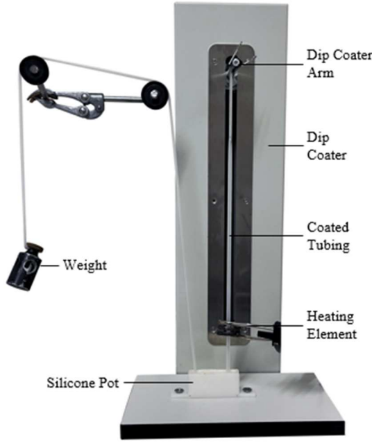
Fig. 1. Dip-coating setup for producing silicone vessels. Commercial tubing is pulled through a silicone pot to become coated in the silicone mixture, followed by a heating element to accelerate the curing of the silicone coating. Finally, the inner tubing is removed, leaving the silicone coating as a custom vessel.
