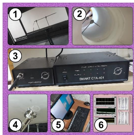
Figure 9- Schematic for Hot-Wire System Arrangement
