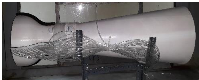
47 Figure 6 - Schematic of the installation of static pressure switches at the inlet contraction wall
