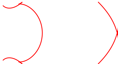
Fig. 11. Examples of undercuts that occur on the inner rotor profiles of a sinusoidal rack generated profile for non-valid regions in Fig. 9(a).
