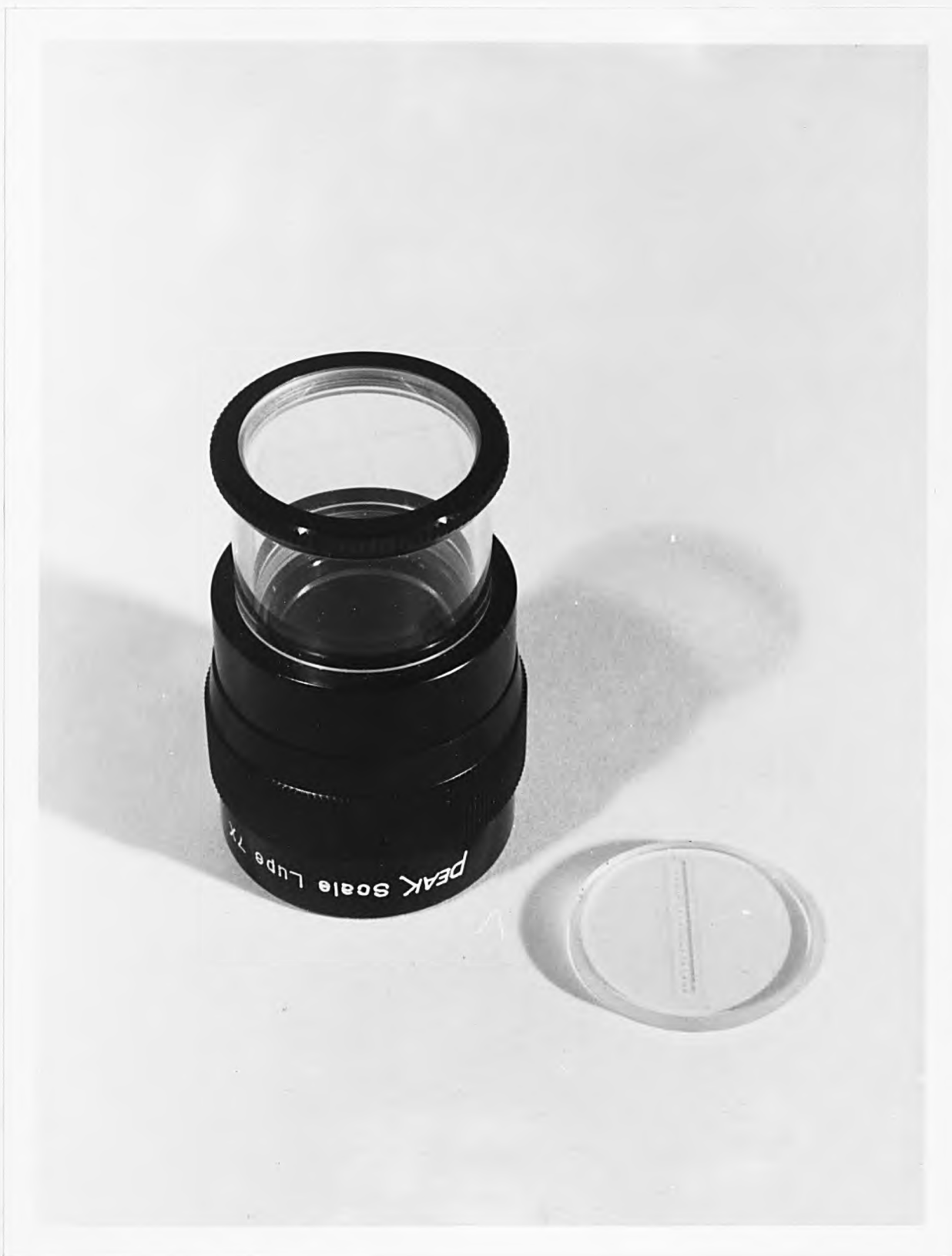
Figure 4.13. Measuring magnifier used for HVID measurements on negatives.
