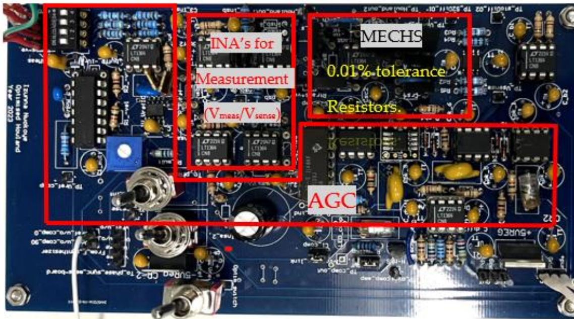
Figure 7.4 Photograph of the AHCS circuit board with the main stages labelled.
