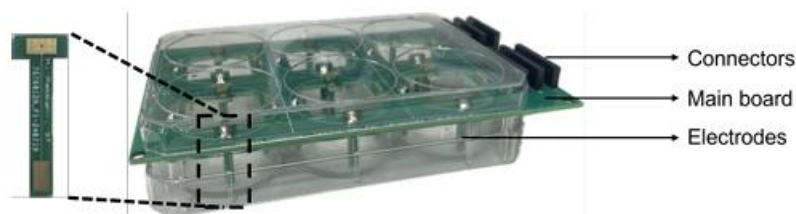
Figure 8.2 PCB electrode setup for the 6-well culture dish
